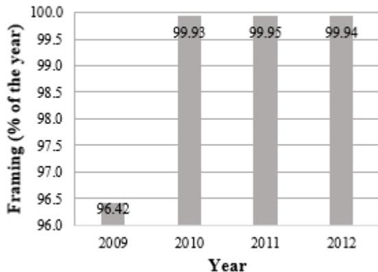
Figure 4. Framing duration of frequency within the normal range of variation: (49.90-50.10) Hz.
