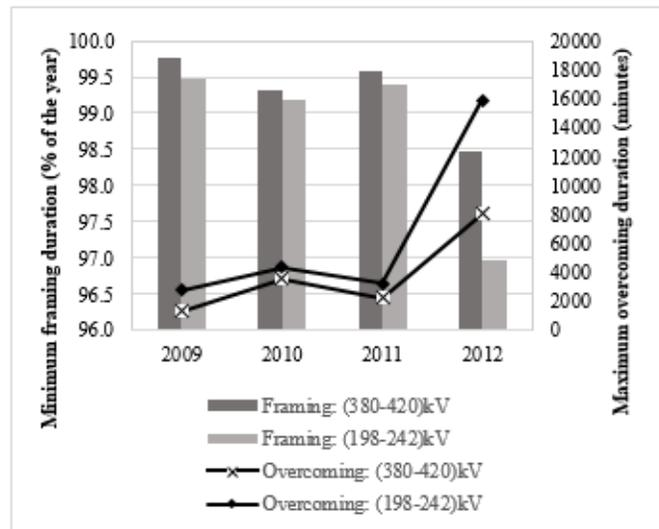
Figure 5. Overcoming the admissible voltage range on voltage levels (220 kV si 400 kV).
