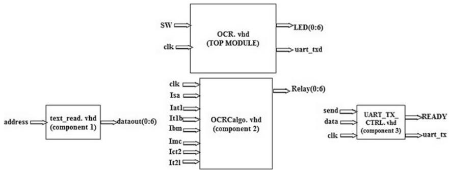
Fig. 2 VHDL modules for OCR coordination algorithm
