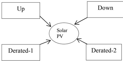
Fig.3 Four-state model of solar PV
