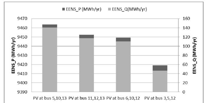
Fig.10 PV locations and EENS for 0.9 Power factor.
