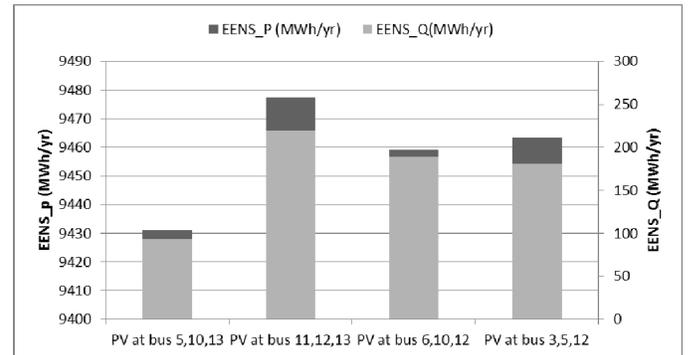
Fig.11 PV locations and EENS for 0.85 Power factor.
