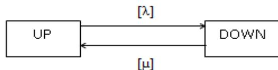
Fig.1 Two-state model for conventional generator
