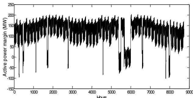
Fig.7 Active power margin without PV
