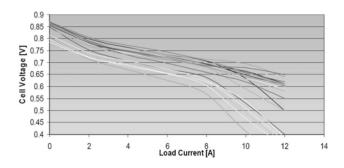
Fig. 3. Individual cell V-I curves for the 12-V, 150-W, 24-cell fuel cell stack.
