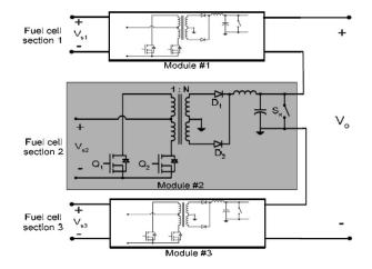
Fig. 9. Proposed modular dc-dc converter.
