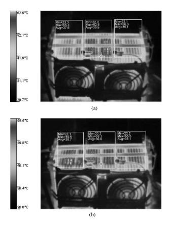
Fig. 14. Thermal comparison of conventional and modular fuel cell.
