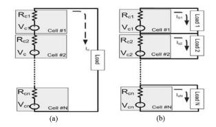
Fig. 5. Modular fuel cell simplified equivalent circuit.
