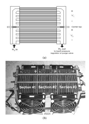
Fig. 6. (a) Schematic drawing of the modular fuel cell stack. (b) Prototype of the 12-V, 150-W, 24-cell modular fuel cell stack.
