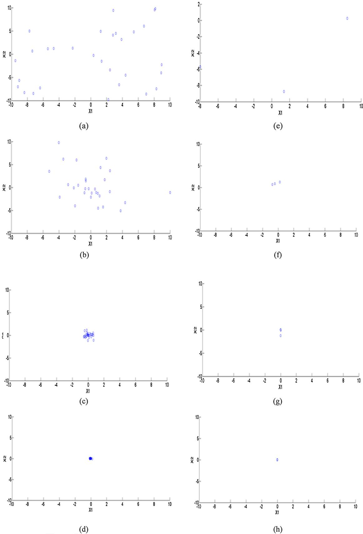
Fig. 17. Population distributions of RLMP SO as compared with PSO, i.e., (a)–(d) distribution of PSO at FEs = 1, 200, 500, and 900; (e)–(h) distribution of RLMP SO at FEs = 1, 200, 500, and 900, respectively.
