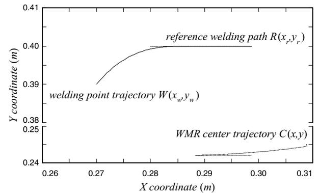
Fig. 9. Trajectories of the WMR and its reference.
