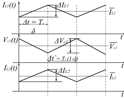
Fig. 3. Cuk converter operation
