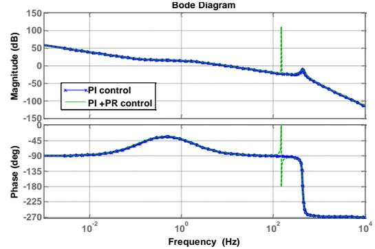
Fig. 10. Impact of the additional control loop
