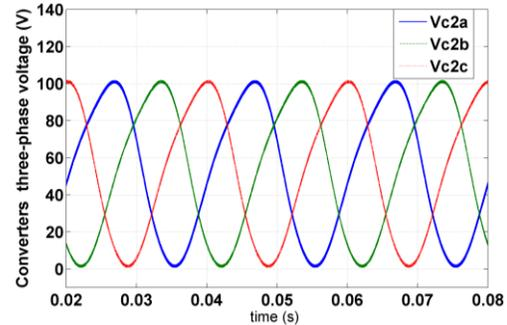
(c) Output voltages at  $V_{c2a}$ ,  $V_{c2b}$  and  $V_{c2c}$
