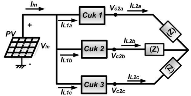
Fig. 2. Proposed Cuk-based three-phase Inverter
