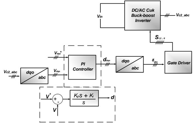
Fig. 6 Control Structure
