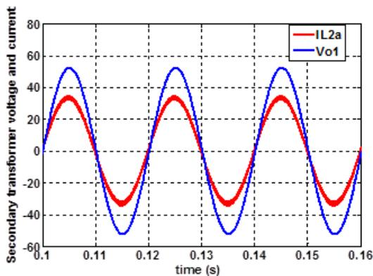
Fig. 13. Secondary voltages and currents
