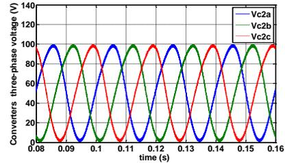
(a) Output voltages at  $V_{c2a}$ ,  $V_{c2b}$  and  $V_{c2c}$  and corresponding  $dq$  components
