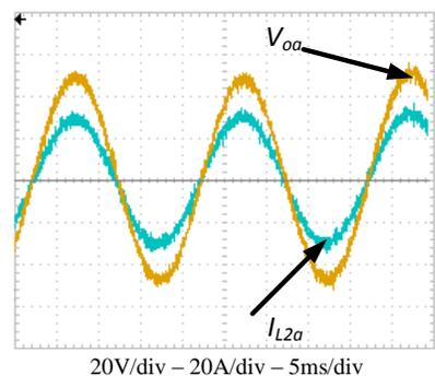
Fig. 17. Secondary voltage and currents
