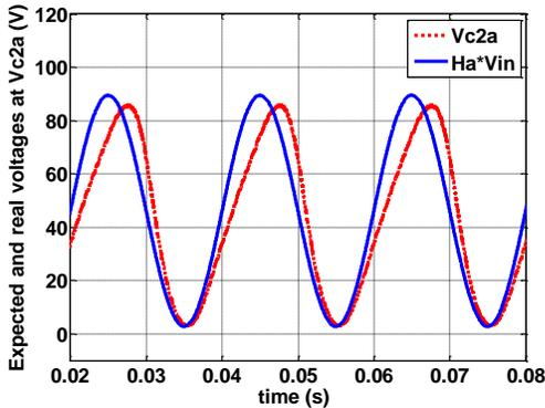
(c) Cuk voltage with time varying duty ratio
