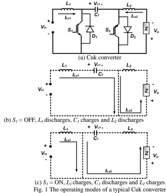
The state space averaging method will be used to model the Cuk converter. Assuming the turn off time of  $S_1$  is  $T_{off}$ , turn on time for  $S_1 = \text{ON}$  is  $T_{on}$  and  $T_s = T_{on} + T_{off}$ , the state space equations during a continuous conduction mode of operation can be written as:
