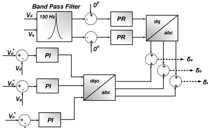
Fig. 9. Control structure with eliminating the 3<sup>rd</sup> harmonic in the  $dq$  frame (2<sup>nd</sup> in the stationary)
