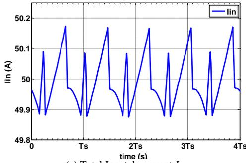
Fig. 12. Reduced high frequency ripples
