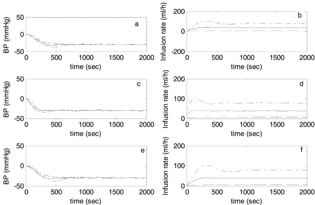
**Fig. 7.** (a), (c) and (e) are the blood pressure (BP) responses and (b), (d) and (f) are SNP drug infusion rate for IMC based TDF-PID, ODF-PI and conventional IMC controller, respectively. (Solid line denotes nominal patient, Dash line denotes sensitive patient, Dash-dot line denotes insensitive patient).
