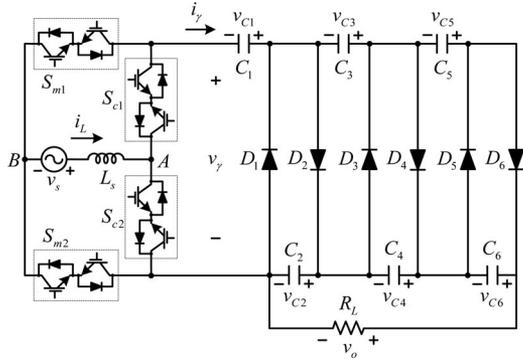
Fig. 3. Proposed converter with a three-stage CW voltage multiplier.
