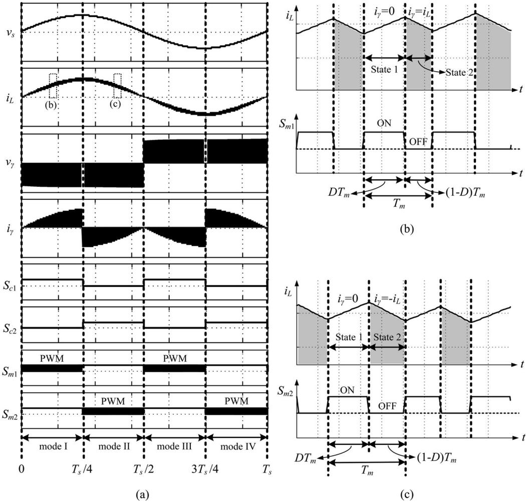
Fig. 6. Some selected waveforms of the proposed converter for illustrating operation modes. (a) Waveforms of  $v_s$ ,  $i_L$ ,  $v_\gamma$ ,  $i_\gamma$ , and trig signals for  $S_{m1}$ ,  $S_{m2}$ ,  $S_{c1}$ , and  $S_{c2}$ . (b) Zoom-in waveforms of  $i_L$  and  $S_{m1}$  at mode I. (c) Zoom-in waveforms of  $i_L$  and  $S_{m2}$  at mode II.
