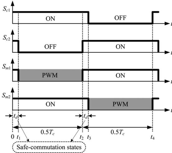
Fig. 8. Timing diagram of switching pattern for the proposed converter including safe-commutation states.
