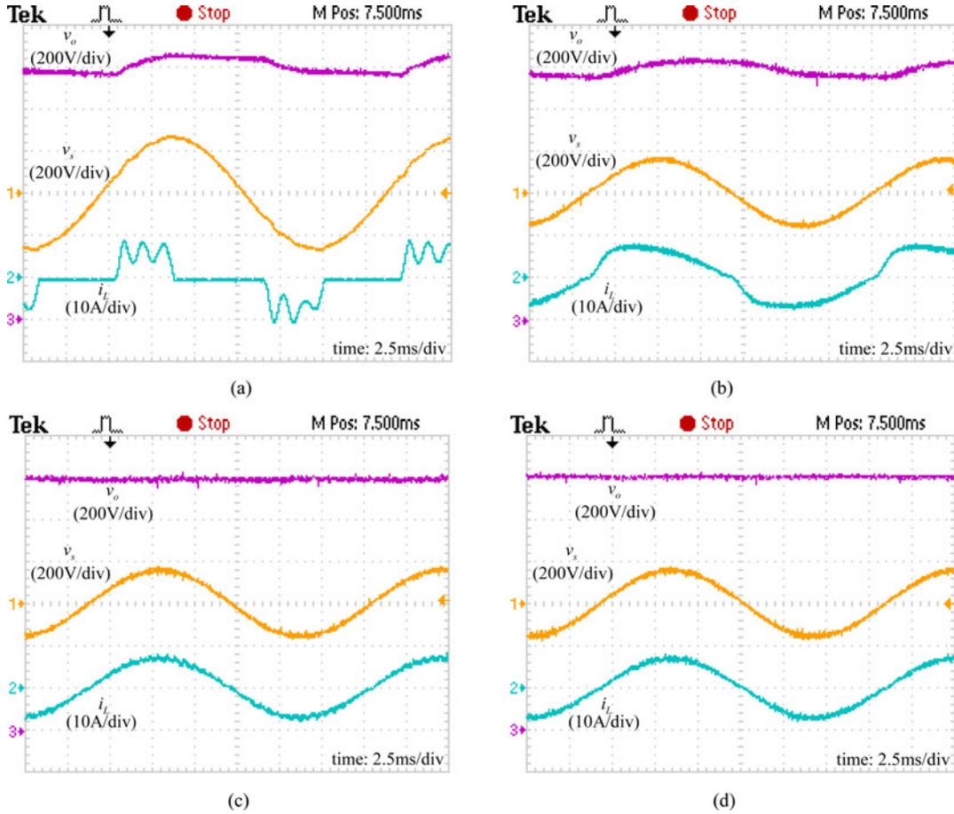
Fig. 12. Experimental waveforms of  $v_s$ ,  $i_L$ , and  $v_o$  at full-load condition. (a) Conventional CW circuit. (b)–(d) Proposed converter with  $f_c = 60$ , 960, and 1920 Hz, respectively.
