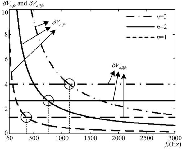
Fig. 11. Normalized output voltage ripple versus alternating frequency with different stages of CW circuit.
