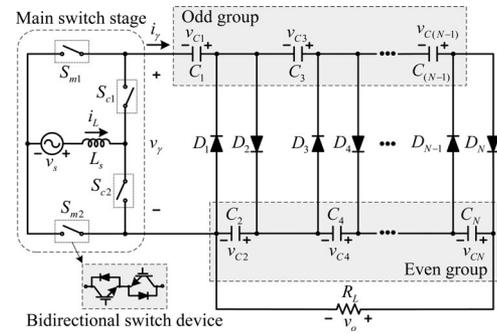
Fig. 2. Circuit configuration of the proposed converter.
