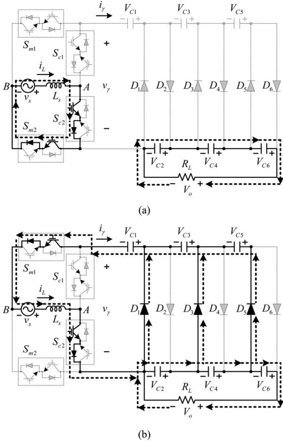
Fig. 5. Circuit states and conducting paths of the proposed converter at mode II. (a) State 1. (b) State 2.
