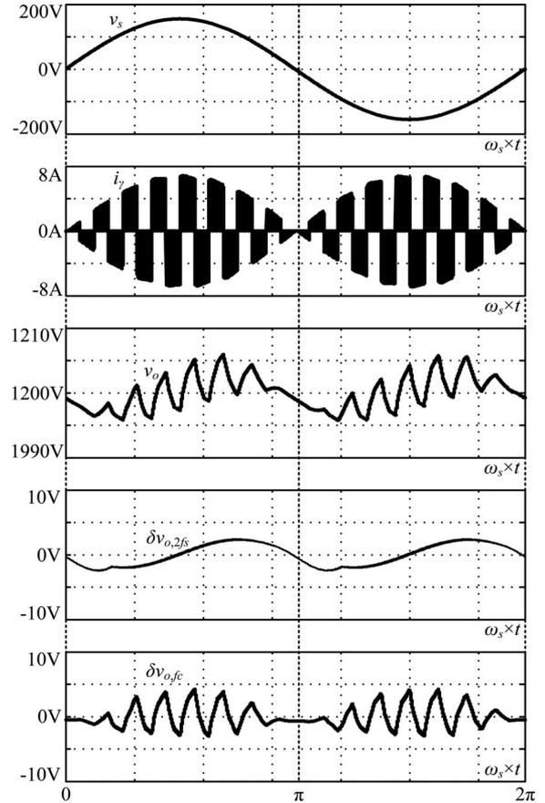
Fig. 10. Simulated waveforms of  $v_s$ ,  $i_\gamma$ ,  $v_o$ ,  $v_o$ ,  $\delta v_{o,2f_s}$ , and  $\delta v_{o,f_c}$  with  $f_c = 960$  Hz and  $P_o = 500$  W.
