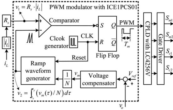
Fig. 9. Control scheme of the proposed converter.
