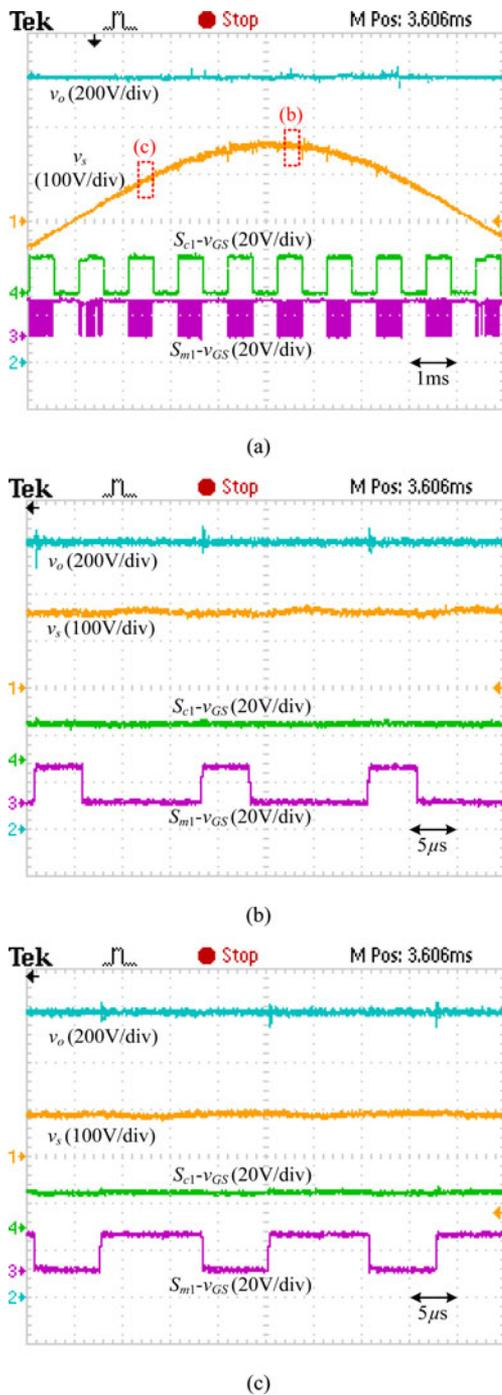
Fig. 16. (a) Experimental waveforms of  $v_o$ ,  $v_s$ ,  $S_{c1-v_{GS}}$ , and  $S_{m1-v_{GS}}$  when  $P_o = 400$  W,  $V_s = 110$  V<sub>rms</sub>,  $V_o = 1.2$  kV, and  $f_c = 960$  Hz during positive-half cycle of input line source. (b) Zoom-in waveforms of area b ( $v_s = 155$  V). (c) Zoom-in waveforms of area c ( $v_s = 80$  V).
