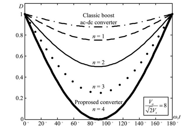
Fig. 7. Duty cycle varying within positive- or negative-half cycles of the line source  $v_s$  for the proposed converter with  $n = 1-4$  and classic boost ac–dc converter.
