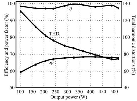
Fig. 14. Experimental results of efficiency, power factor, and THD of the conventional CW circuit under different load conditions.
