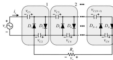
Fig. 1. Conventional  $n$ -stage CW voltage multiplier.
