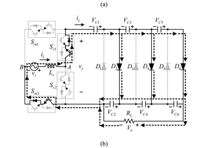
Fig. 4. Circuit states and conducting paths of the proposed converter at mode I. (a) State 1. (b) State 2.
