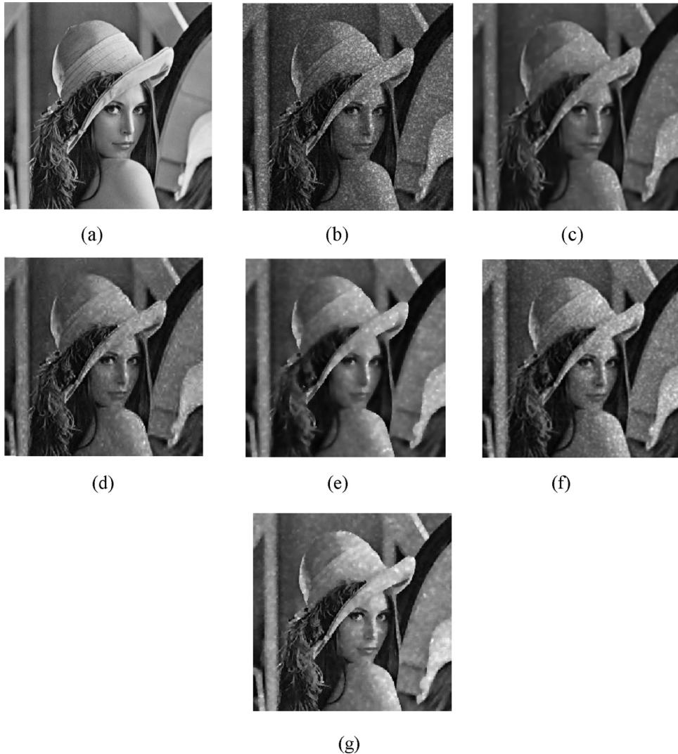
**Fig. 4.** Comparison of various despeckling methods. (a) Noise free Lena image, (b) noisy image of noise standard deviation 0.7. Denoised image obtained by using (c) GenLik [10], (d) SNIG I [11], (e) adaptive bilateral filter [12], (f) ATMAV [16], and (g) proposed adaptive fuzzy logic filter based on CV.
