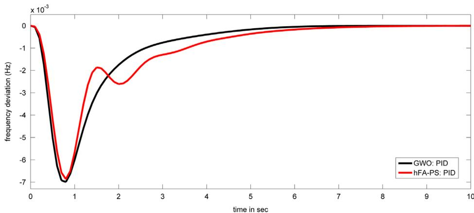
**Fig. 12.** Changes of frequency with 1.5% SLP in area-1 for test system-2.
