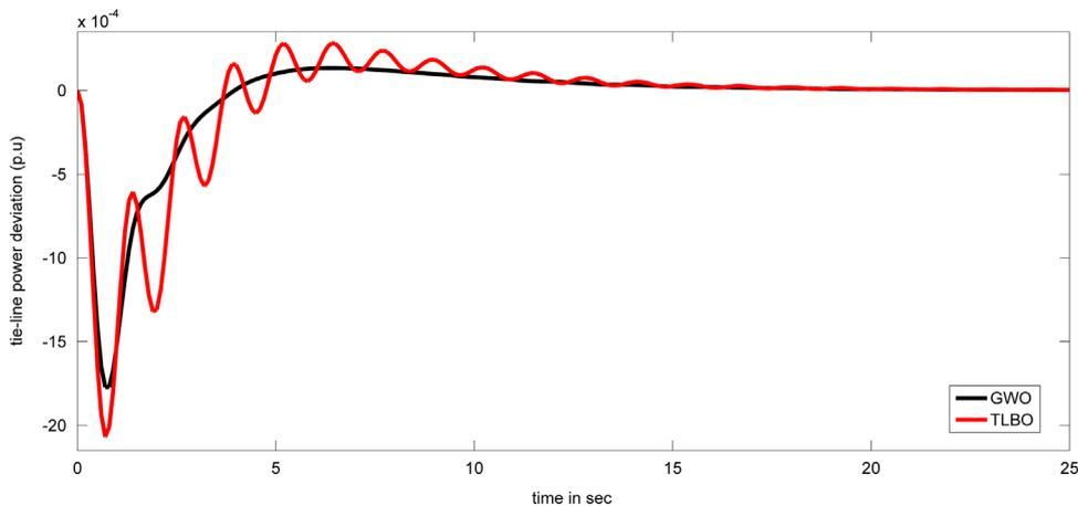
Fig. 15. Changes of tie-line power with 1% SLP in area-1 for test system-3 considering AC tie-line only.
