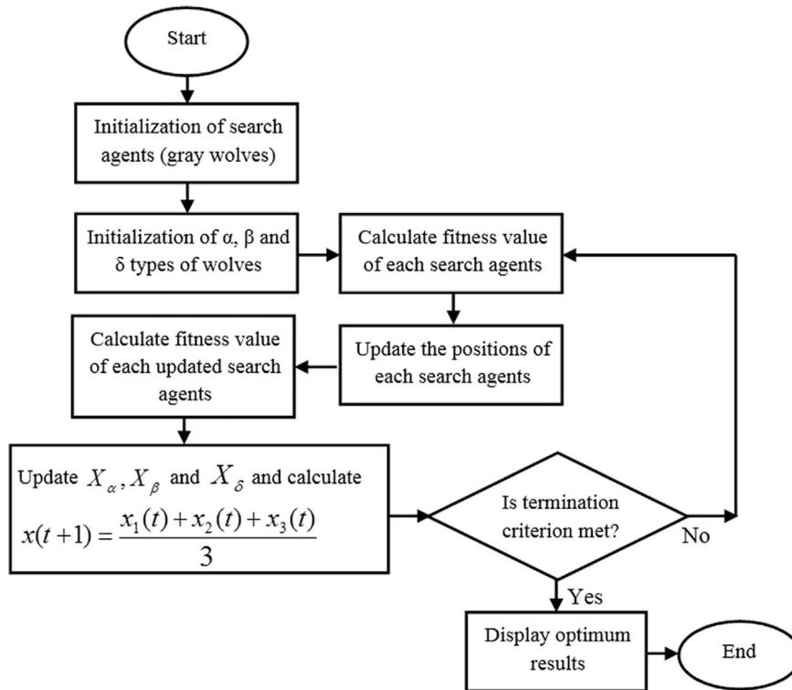
Fig. 2. Flowchart of GWO-algorithm.
