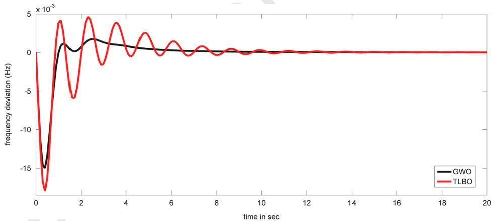
Fig. 14. Changes of frequency with 1% SLP in area-1 for test system-3 considering AC tie-line only.
