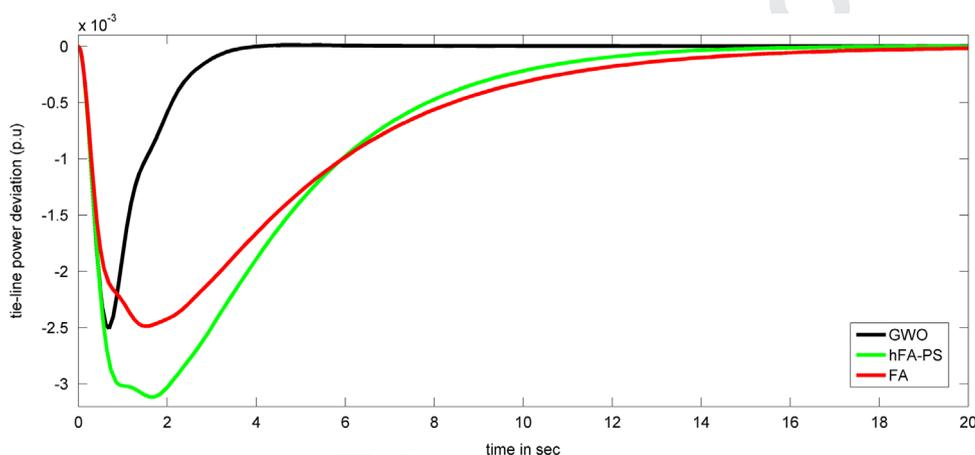
Fig. 10. Changes of tie-line power with 5% SLP in area-1 considering 0.025 GRC for test system-1
