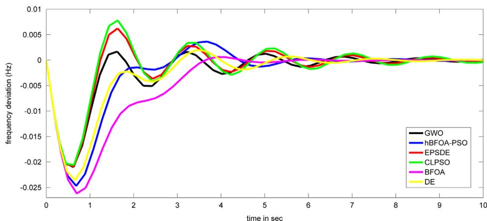
Fig. 3. Changes of frequency with 10% SLP in area-1 for test system-1.
