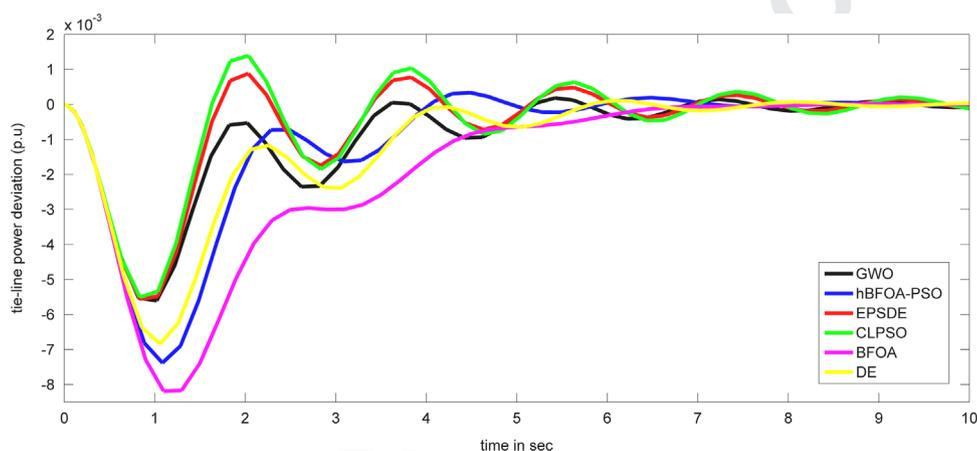
Fig. 4. Changes of tie-line power with 10% SLP in area-1 for test system-1.
