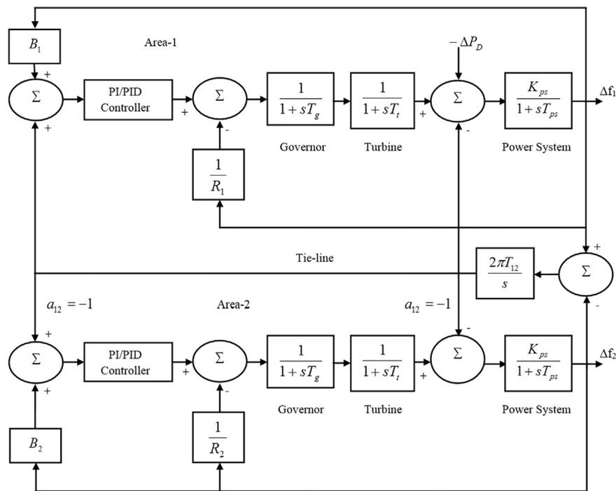
Fig. 1. Block diagram of two-area interconnected non-reheat thermal-thermal power system (test system-1).
