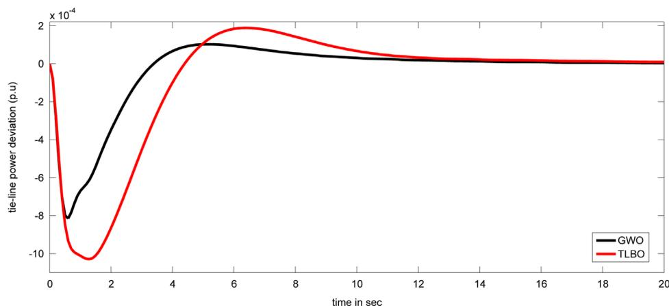
Fig. 17. Changes of tie-line power with 1% SLP in area-1 for test system-3 considering AC-DC tie-line.
