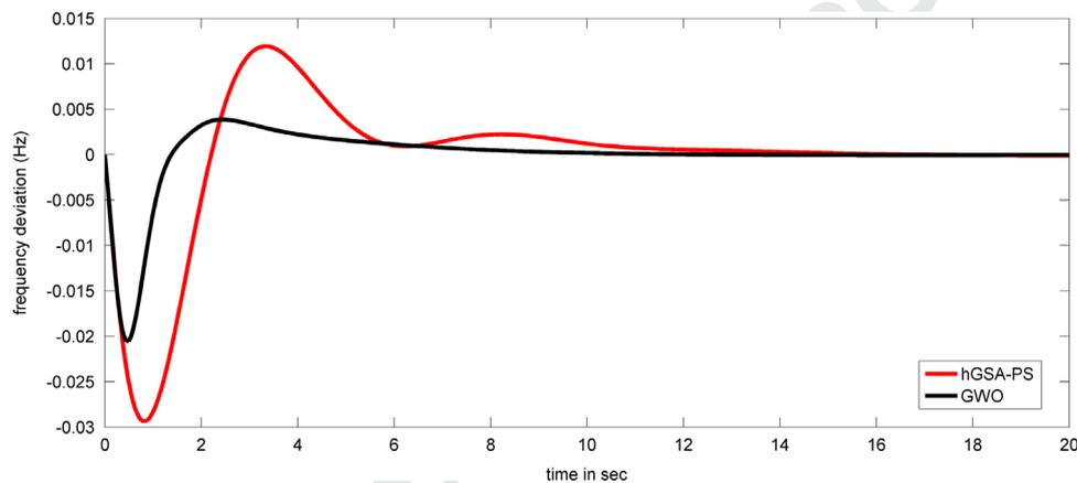
Fig. 20. Changes of frequency with PID-controller after 1% SLP in area-1 for test system-4.
