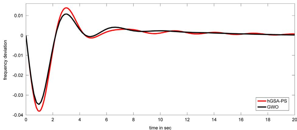
**Fig. 18.** Changes of frequency with PI-controller after 1% SLP in area-1 for test system-4.
