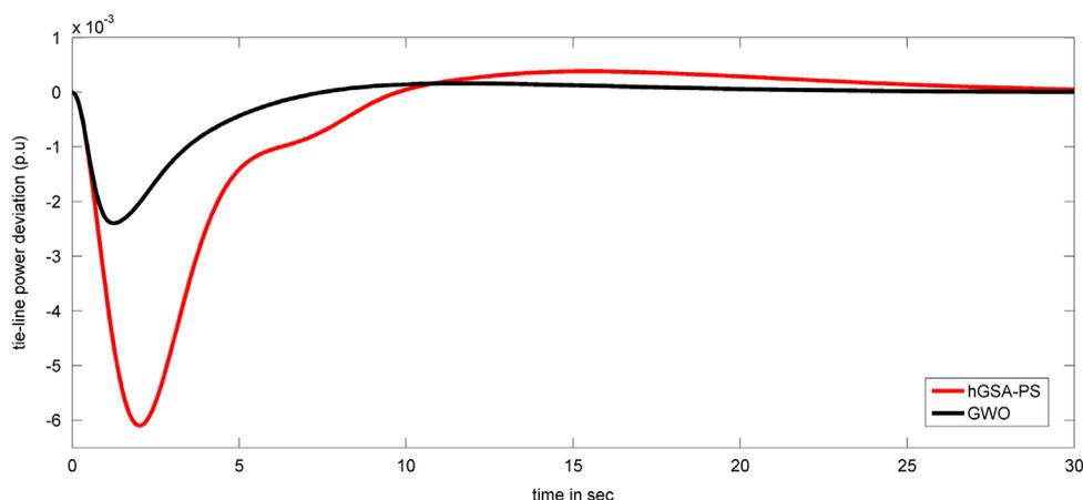
Fig. 21. Changes of tie-line power with PID-controller after 1% SLP in area-1 for test system-4.
