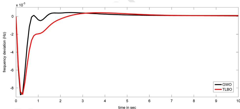
Fig. 16. Changes of frequency with 1% SLP in area-1 for test system-3 considering AC-DC tie-line.
