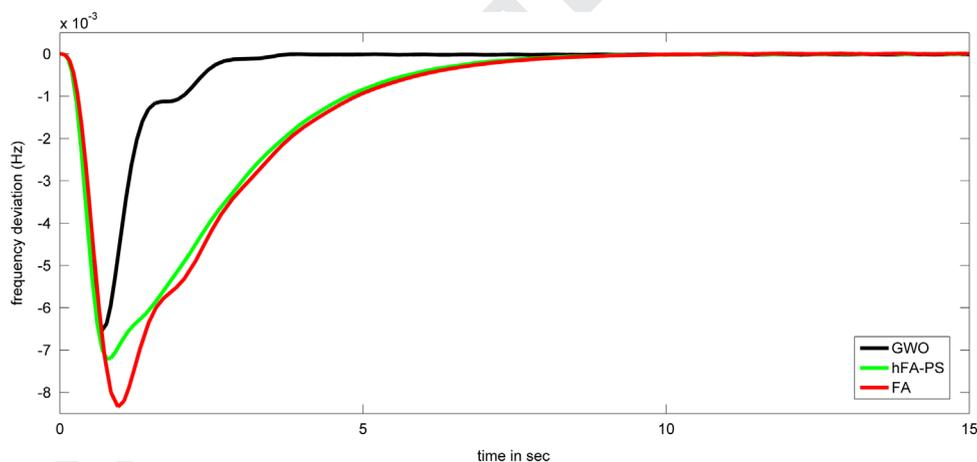
Fig. 7. Changes of frequency with 5% SLP in area-1 considering 0.05 GRC for test system-1.
