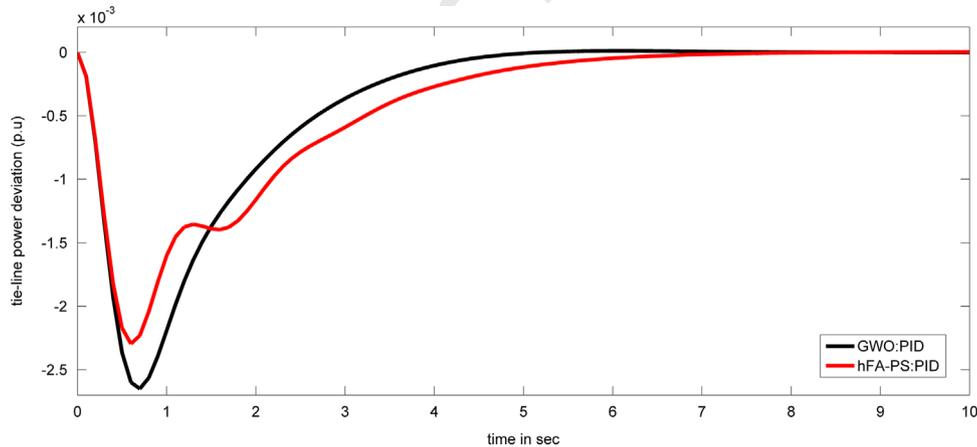
Fig. 13. Changes of tie-line power with 1.5% SLP in area-1 for test system-2.
