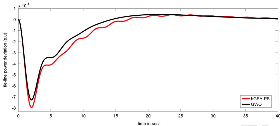
Fig. 19. Changes of tie-line power with PI-controller after 1% SLP in area-1 for test system-4.
