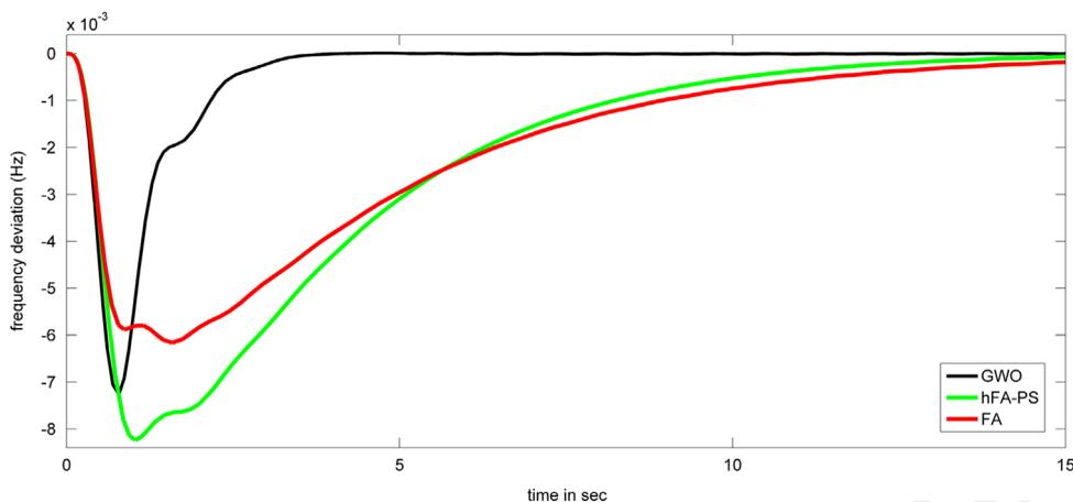
Fig. 9. Changes of frequency with 5% SLP in area-1 considering 0.025 GRC for test system-1.
