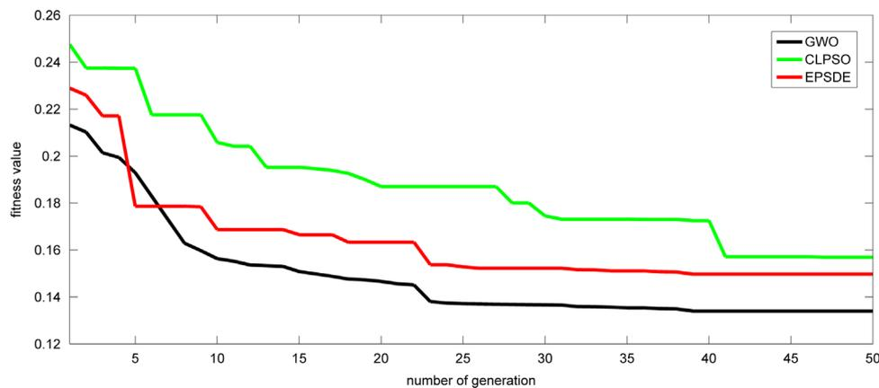
Fig. 6. Convergence profile of proposed algorithms for test system-1 with PID-controller structure.
