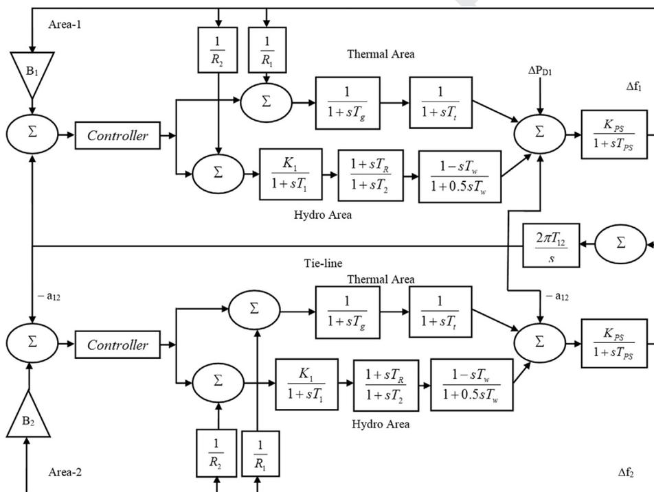
**Fig. 11.** Block diagram of two-area interconnected multi-units hydro-thermal power system (test system-2).
