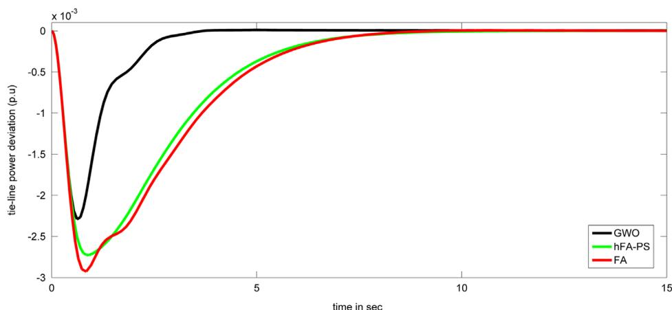
Fig. 8. Changes of tie-line power with 5% SLP in area-1 considering 0.05 GRC for test system-1.
