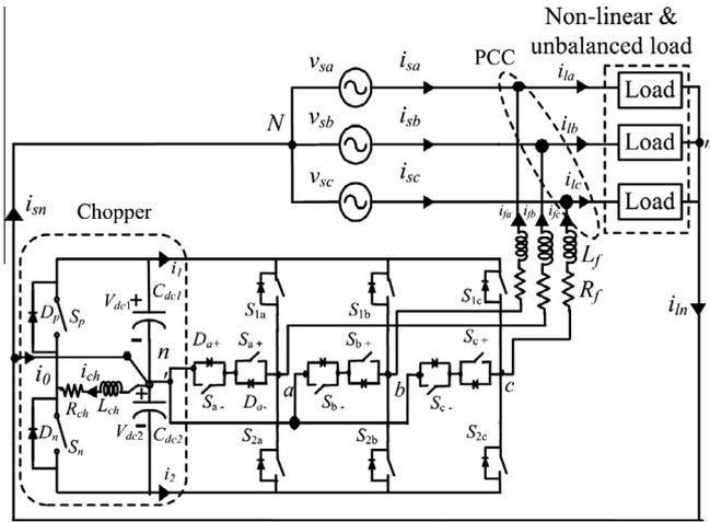
Fig. 3. DSTATCOM using MNPC inverter.
