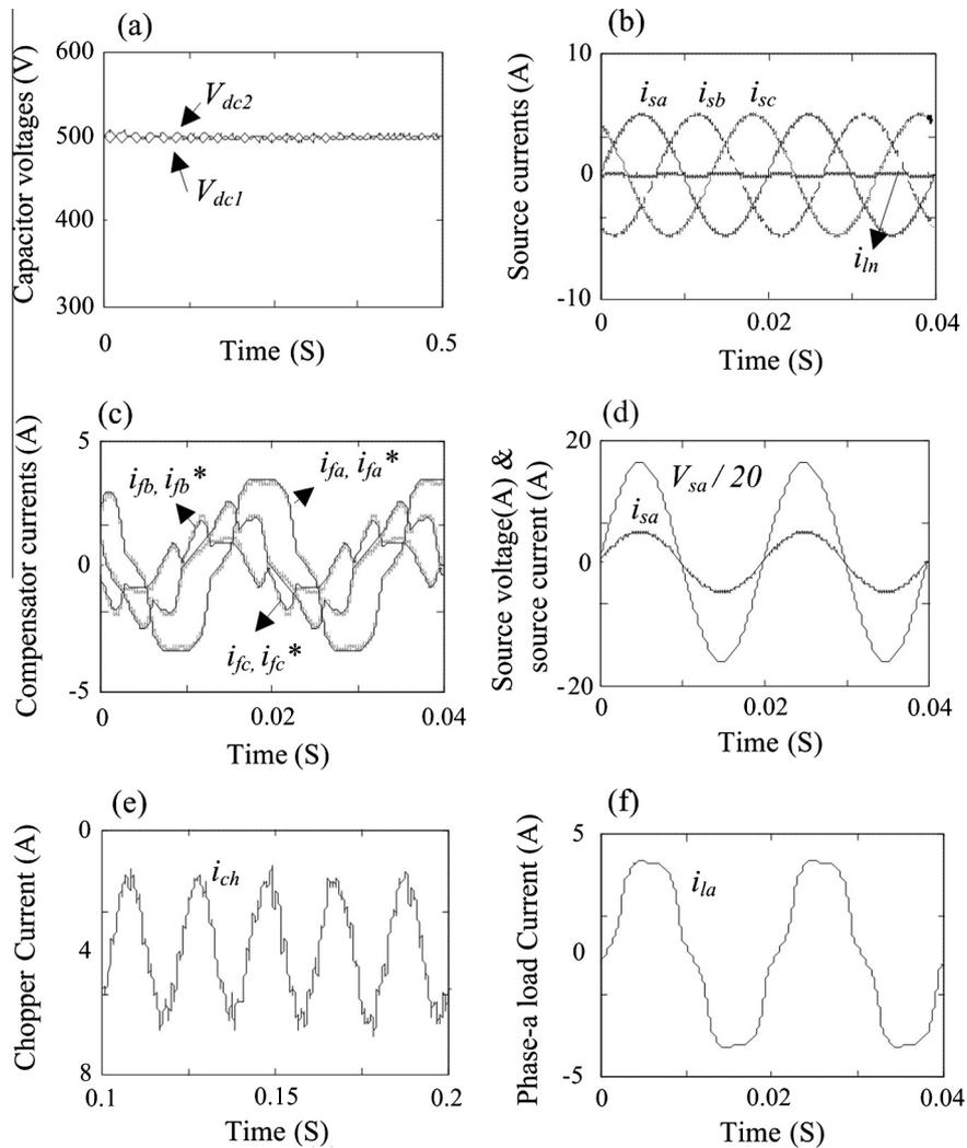
**Fig. 8.** Simulation results after compensation using CNPC DSTATCOM with capacitor balancing (a) capacitor voltages (b) source currents (c) compensator and reference injected currents (d) source voltage and source current (phase-a) (e) chopper current (f) phase-a load current.
