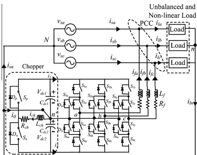
Fig. 4. DSTATCOM using ANPC inverter.
