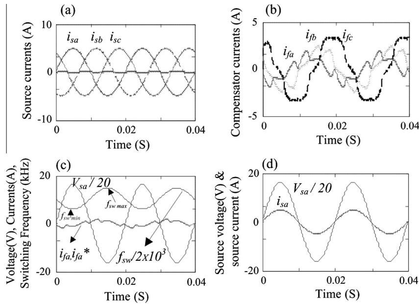
**Fig. 10.** Simulation results with Active NPC DSTATCOM (a) source currents (b) DSTATCOM injected currents (c) source voltage, injected current, reference current and switching frequency (d) source voltage and source currents (phase-a).
