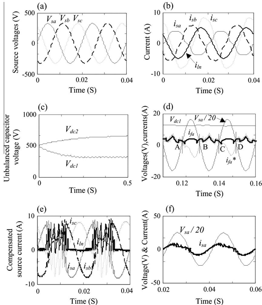
**Fig. 7.** Simulation results after compensation using CNPC without capacitor balancing (a) source voltages (b) source currents (c) capacitor voltages (d) loss of tracking (phase-a) (e) poor source current compensation (f) source voltage and source current.
