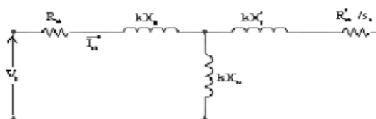
Fig.1 K^{th} harmonic equivalent circuit of induction motor
