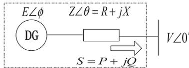
Fig. 1. Equivalent circuit of a microsource.
