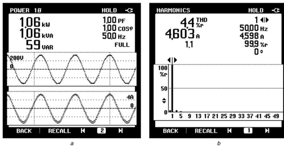
Fig. 9 Output current harmonics, power and the power factor values of inverter
