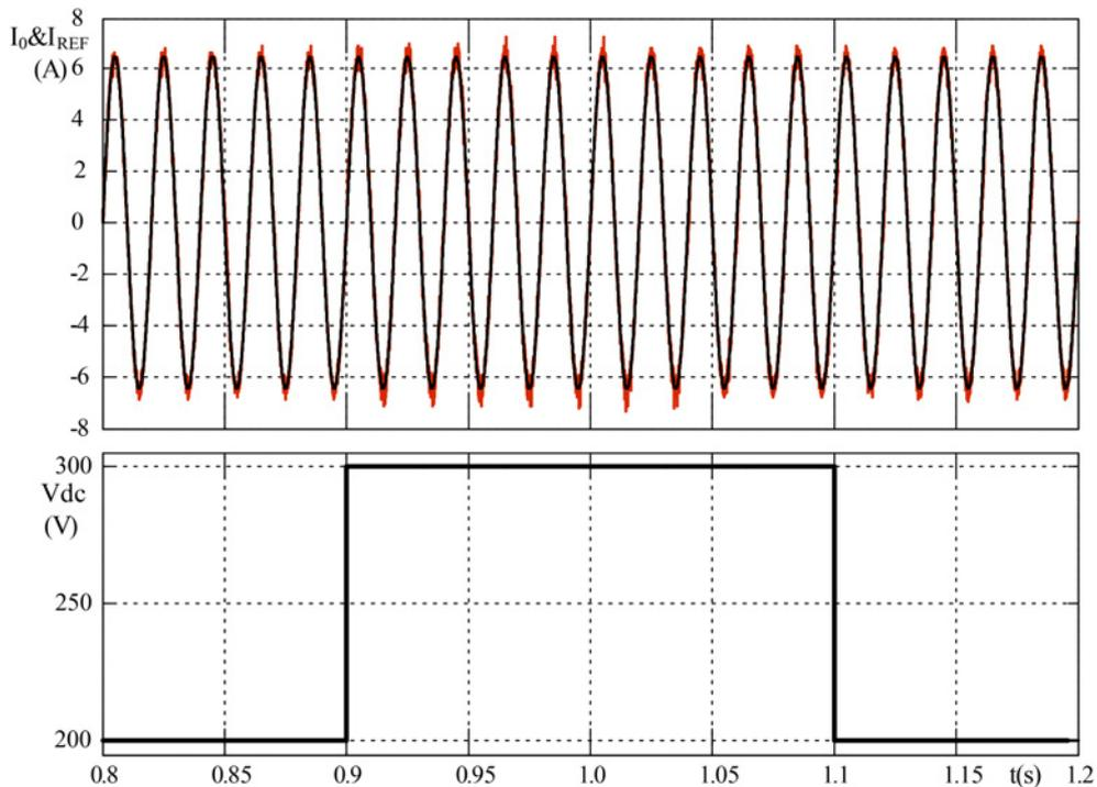
**Fig. 6** Inverter output current and reference current under input DC voltage variations
