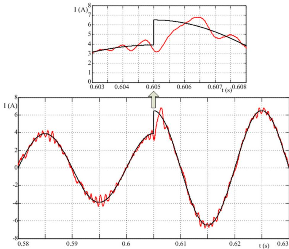
**Fig. 5** Inverter output current and reference current
