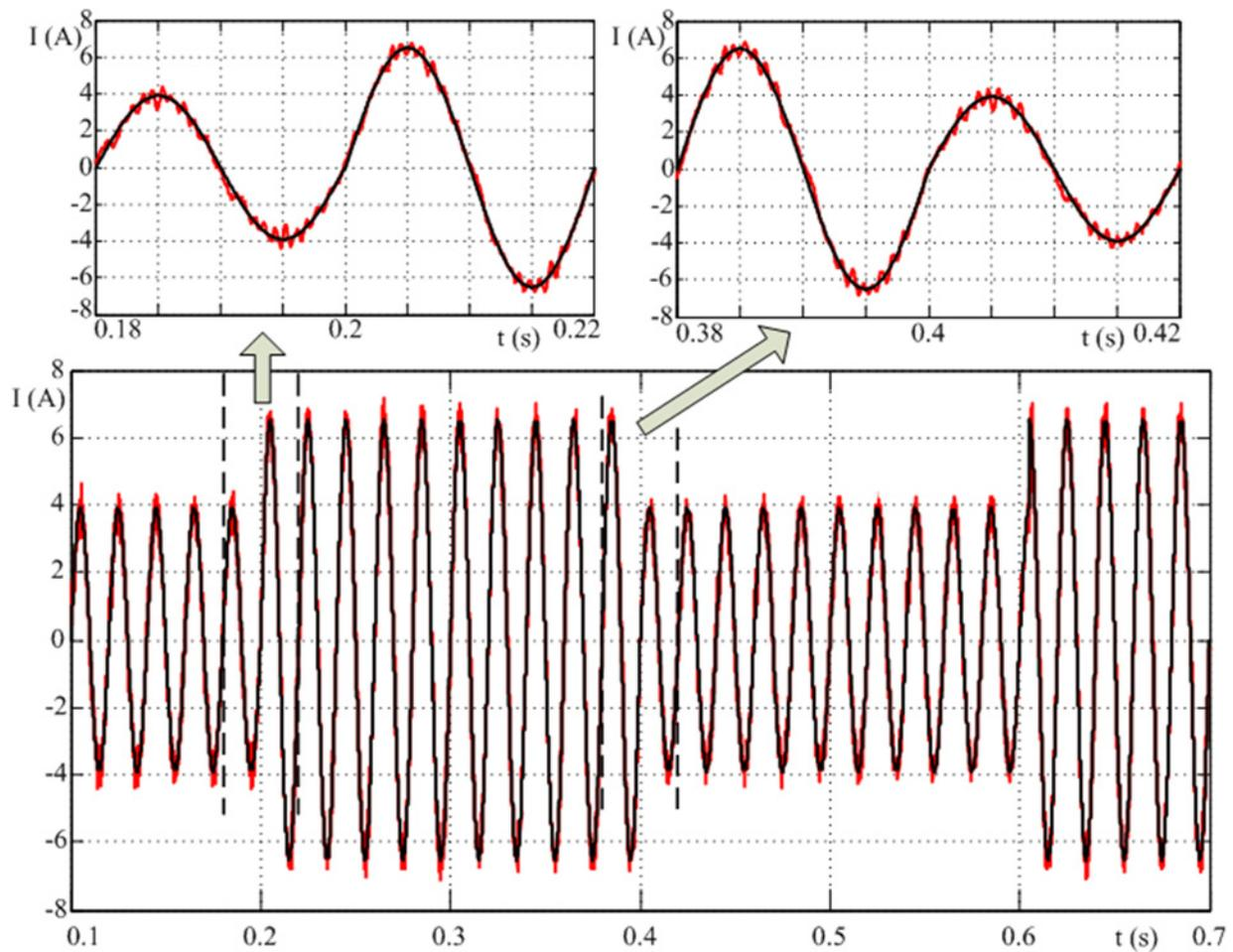
Fig. 4 Inverter output current and reference current
