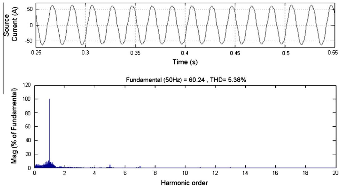
Fig. 9d. Source current for phase A with its spectrum after compensation.
