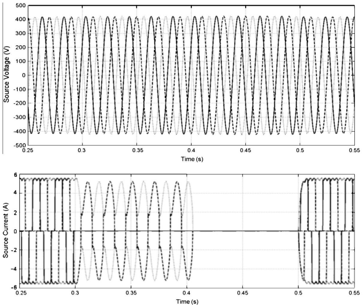
Fig. 9a. Performance of source voltage and source current without compensation.
