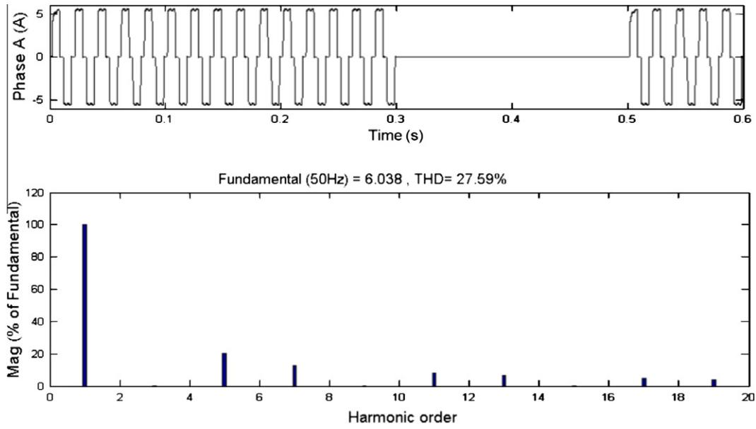
Fig. 9b. Performance of phase A load current with its spectrum without compensation.
