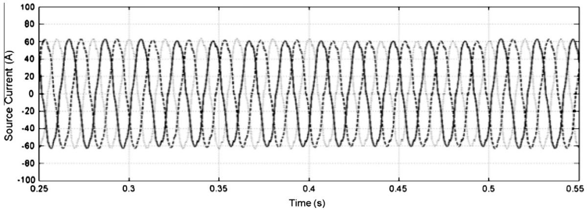
Fig. 9c. Source current after compensation.
