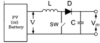
Fig. 7. Topology of PV or battery operated boost converter.
