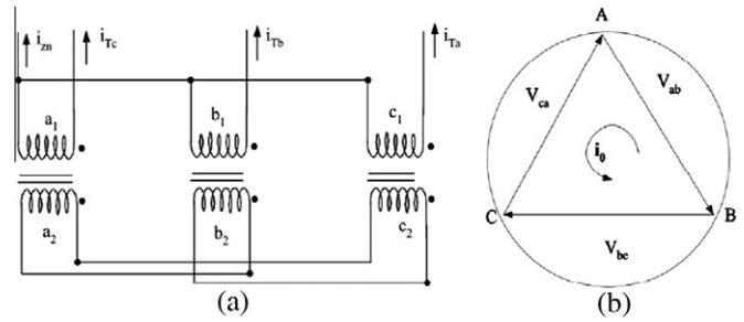
Fig. 2. (a) Star/delta transformer windings. (b) Phasor diagram.
