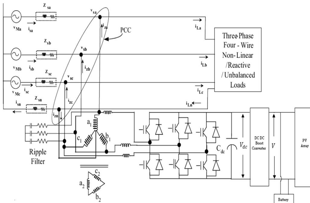
Fig. 1. Schematics of proposed renewable based three-leg VSC with star/delta transformer.
