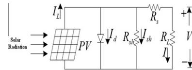
Fig. 3. Equivalent electrical circuit of PV cell.
