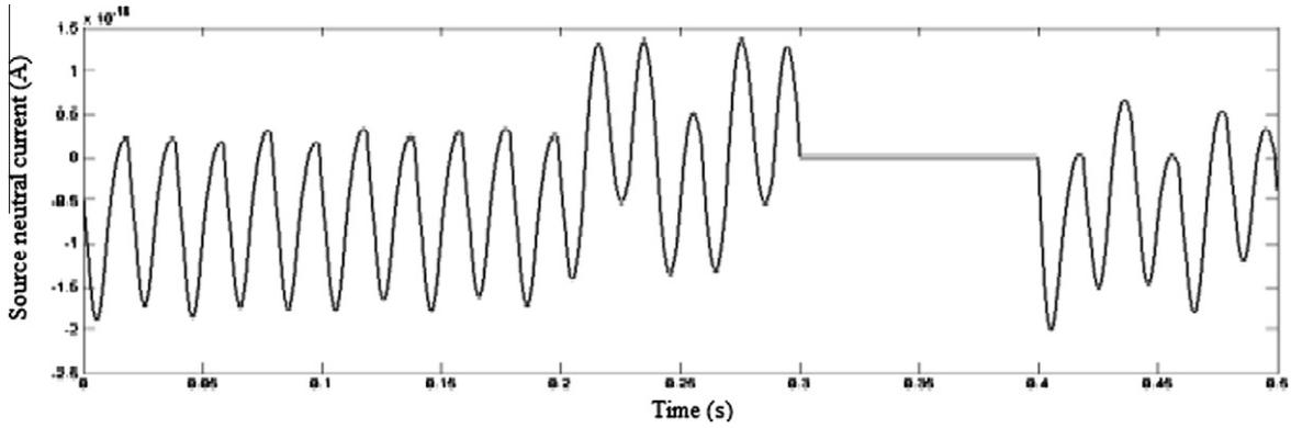
Fig. 9e. Source neutral current after compensation.
