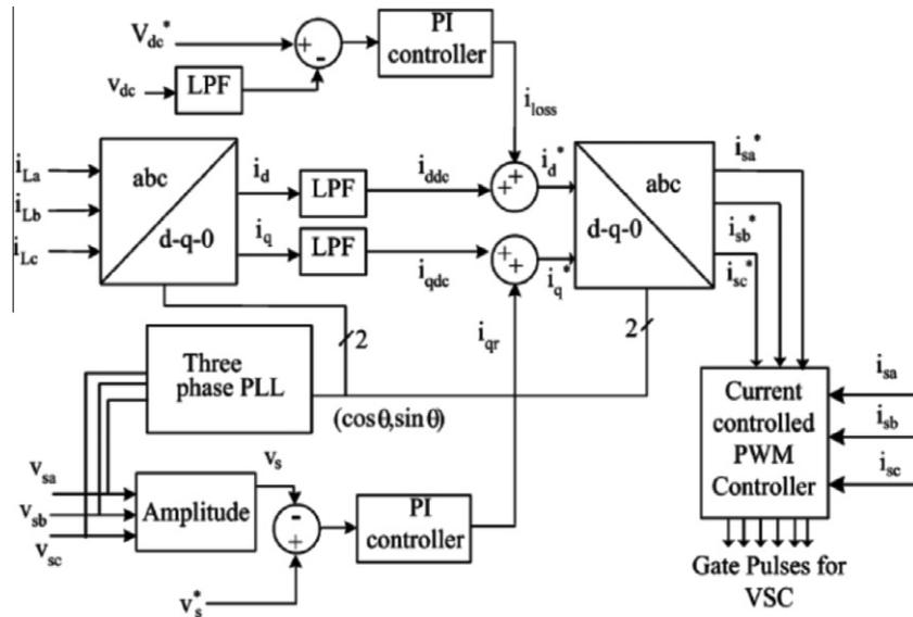
Fig. 8. Control algorithm of three leg VSC.
