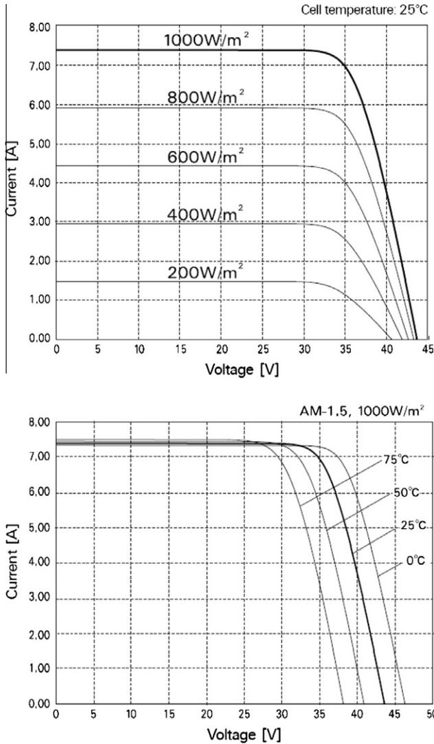
Fig. 6.  $I$ - $V$  characteristics of SANYO-240HDE4 PV Module.
