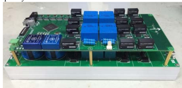
Fig. 10. A single phase circuit of the prototype
