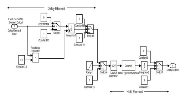
Figure 7. Modeling of Delay Element and Hold Element on SIMULINK®
