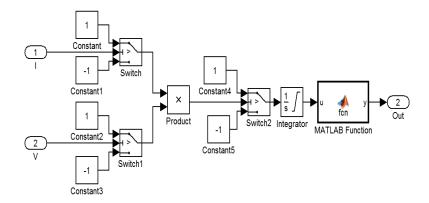
Figure 6. Modelling of Directional Element on SIMULINK
