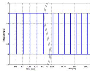
Figure 11. Integrator Input (From Switch2 in directional element)
