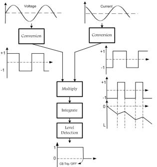
Figure 5. Concept Diagram for Implementing Directional Element.
