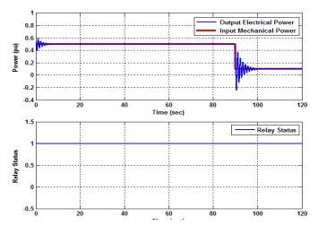
Figure 10. Relay performance (a) Input/Output Power (b) Relay Status
