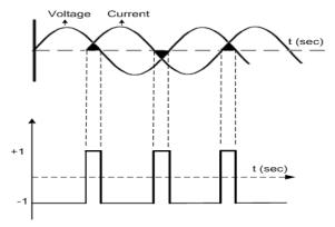
Figure 3b. Angle between Voltage and Current Waveforms under Fault Conditions
