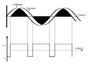
Figure 3a. Angle between Voltage and Current Waveforms under Normal Conditions
