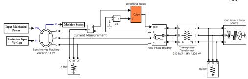
Figure 8. Reverse power relay model in power system
