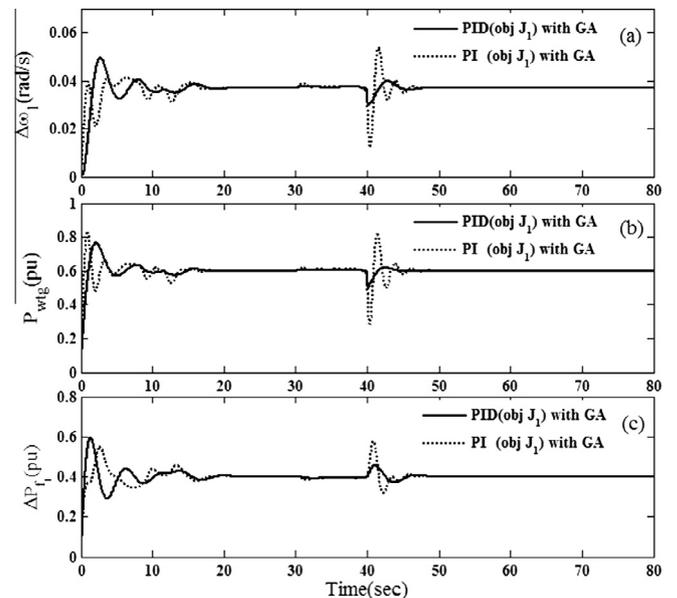
Fig. 5. Dynamic responses for (a) WTG frequency deviation, (b) WTG power output and (c) diesel generator power output considering optimum value of P-I and P-I-D gain parameters obtained using GA (Table 1).
