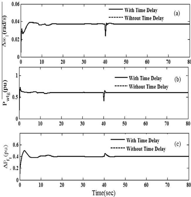
**Fig. 12.** Comparison of dynamic responses for (a) WTG frequency deviation, (b) WTG power output and (c) diesel generator power output, with and without time delay incorporation considering optimum value of P–I–D gain parameters optimized by PSO using fitness function given by Eq. (30).
