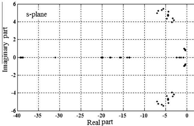
**Fig. 13.** Eigenvalues of wind diesel system with parameter variations.
