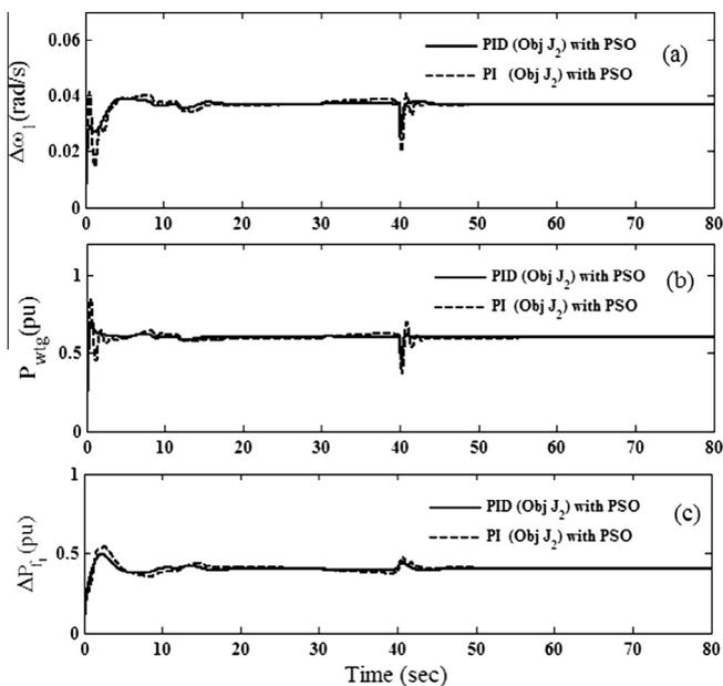
Fig. 9. Dynamic responses for (a) WTG frequency deviation, (b) WTG power output and (c) diesel generator power output considering optimum value of P–I and P–I–D gain parameters using PSO (Table 6).
