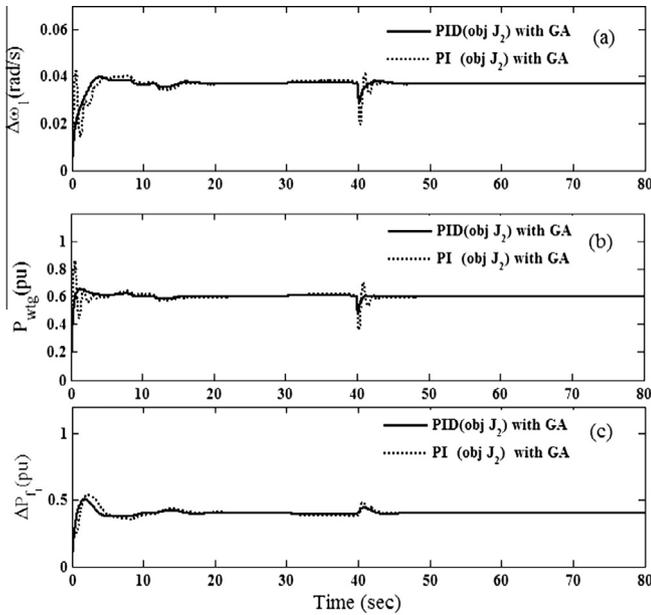
Fig. 6. Dynamic responses for (a) WTG frequency deviation, (b) WTG power output and (c) diesel generator power output considering optimum value of P–I and P–I–D gain parameters obtained using GA (Table 2).
