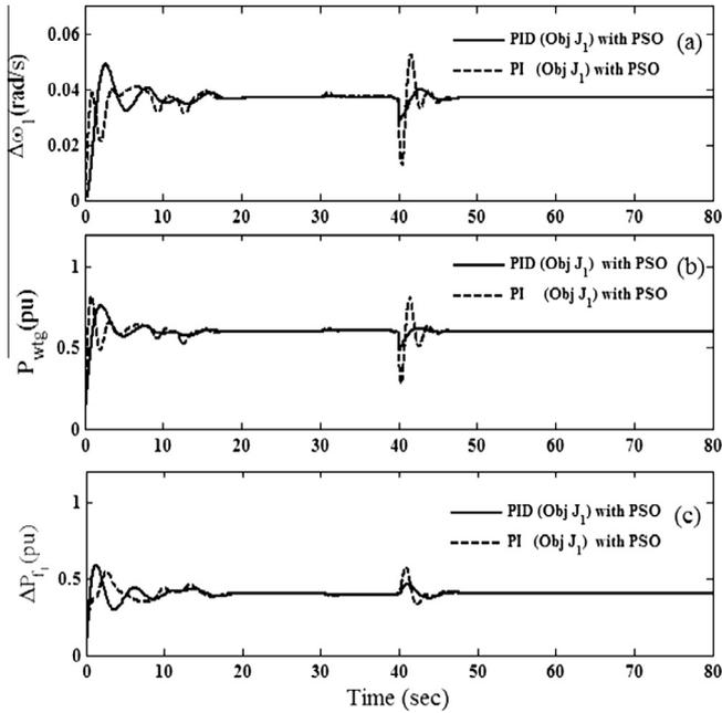
Fig. 8. Dynamic responses for (a) WTG frequency deviation, (b) WTG power output and (c) diesel generator power output considering optimum value of P–I and P–I–D gain parameters using PSO (Table 5).
