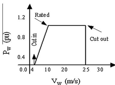
Fig. 1. Wind speed versus wind power.
