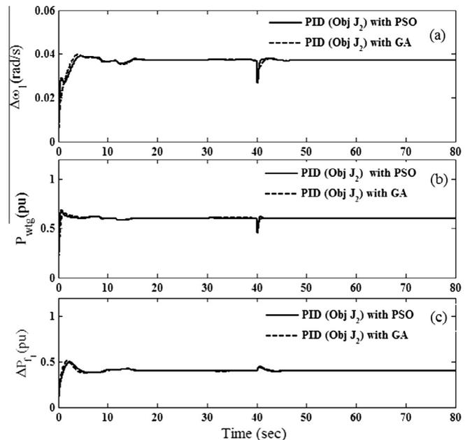
Fig. 11. Comparison of dynamic responses for (a) WTG frequency deviation, (b) WTG power output and (c) diesel generator power output considering optimum value of P–I–D gain parameters optimized by PSO and GA using fitness function given by Eq. (30).
