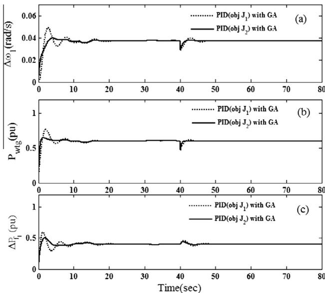
Fig. 7. Dynamic responses for (a) WTG frequency deviation, (b) WTG power output and (c) diesel generator power output considering optimum value of P–I–D gain parameters optimized by GA using fitness functions given by Eqs. (28) and (30).
