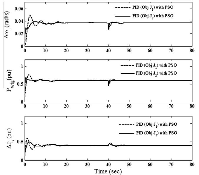
Fig. 10. Dynamic responses for (a) WTG frequency deviation, (b) WTG power output and (c) diesel generator power output considering optimum value of P–I–D gain parameters optimized by PSO using fitness functions given by Eqs. (28) and (30).
