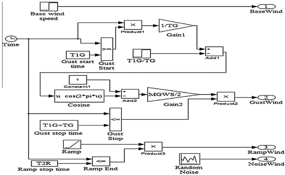
Fig. 4b. Wind speed MATLAB simulink model.
