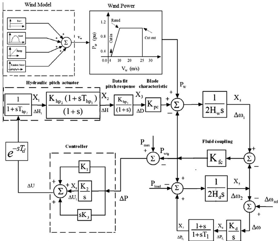
Fig. 3. Wind–diesel small isolated power system.
