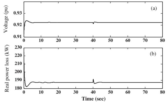
**Fig. 14.** Variations of voltage magnitude of node 61 and real power loss during power injection by wind–diesel hybrid system into the 69 node distribution work.
