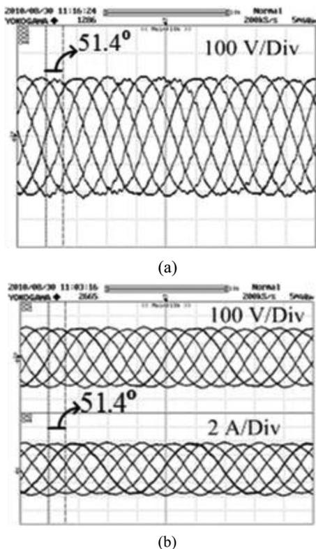
Fig. 8. (a) Seven-phase output voltage waveform (No-load, showing phase difference of  $51.4286^\circ$ ) of the designed transformer secondary. (b) Seven-phase output voltage and current waveforms (loaded, showing phase difference of  $51.4286^\circ$ ) of the designed transformer secondary.
