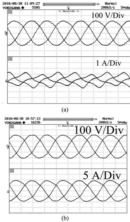
Fig. 7. (a) Input three-phase voltage and current waveforms (no-load) of the designed transformer primary. (b) Input three-phase voltage and current waveforms (loaded) of the designed transformer primary.
