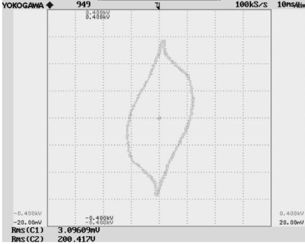
Fig. 9. Lissajous pattern of input voltage versus input current (measured with current probe of 100 mV = 1 A) showing core loss.
