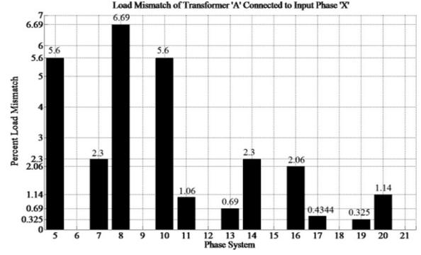
Fig. 5. Load mismatch in different output system of Transformer “A” Connected to input Phase “X.”
