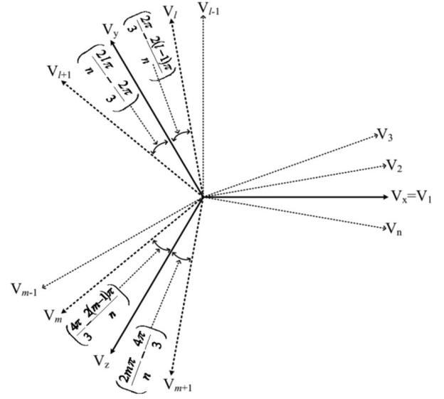
Fig. 4. General Phasor diagram for three-phase system from "n" phase system.
