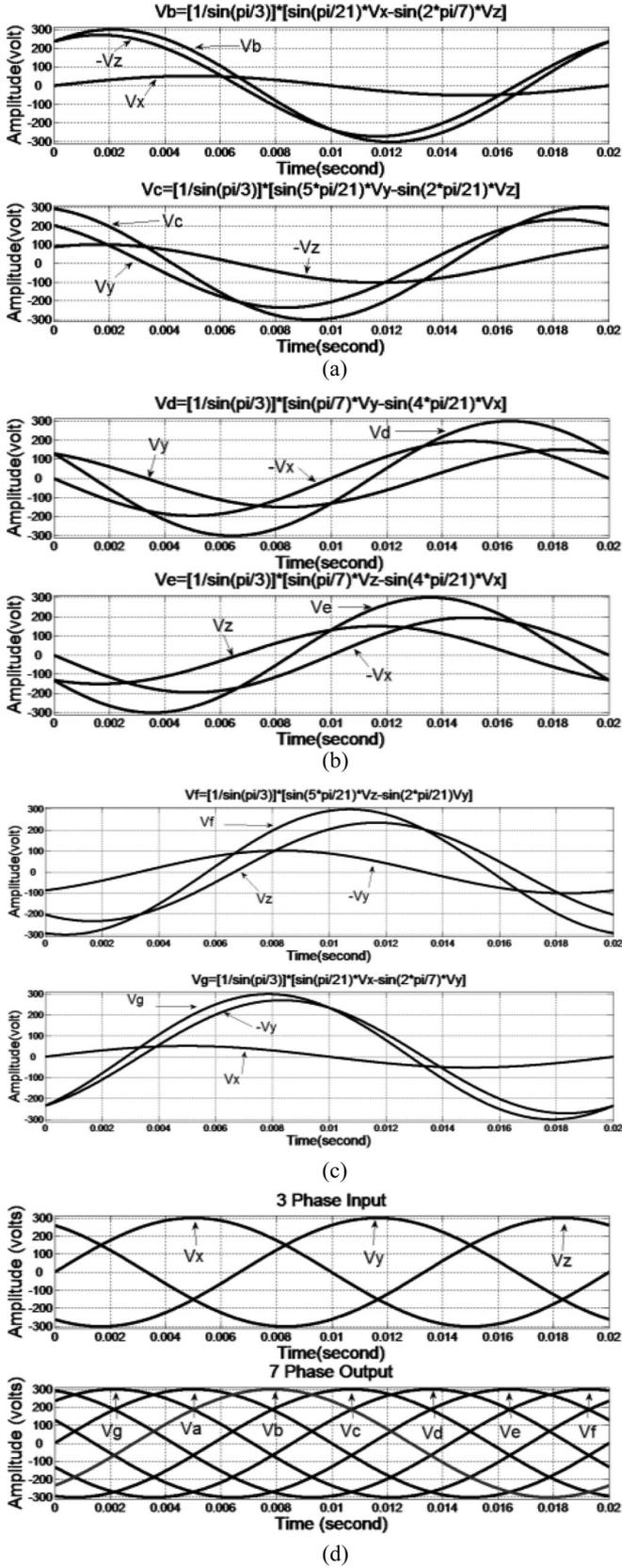
Fig. 6. (a) Input  $V_x$ ,  $V_y$ , and  $V_z$ -phases and output  $V_b$  and  $V_c$  phase voltage waveforms. (b) Input  $V_x$ ,  $V_y$ , and  $V_z$ -phases and output  $V_d$  and  $V_e$  phase voltage waveforms. (c) Input  $V_x$ ,  $V_z$ , and  $V_x$ -phases and output  $V_f$  and  $V_g$  phase voltage waveforms. (d) Simulated three-phase input and seven-phase output voltages.
