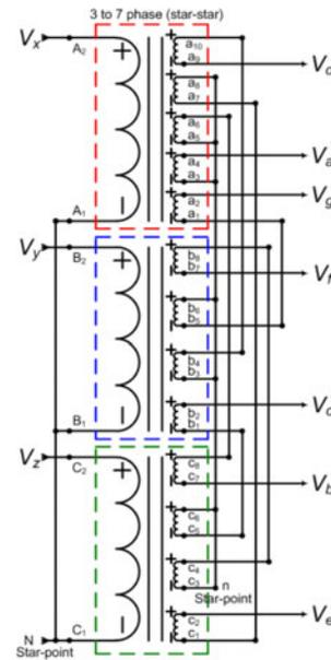
Fig. 2. Proposed transformer winding arrangements (star-star).
