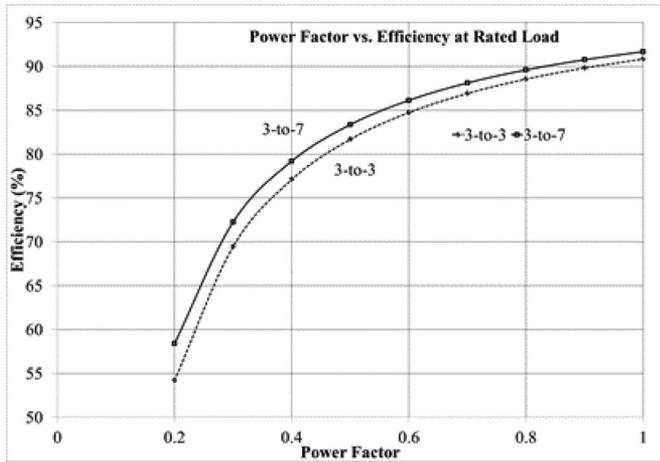
Fig. A.2. Comparison of efficiency of three-to-three and three-to-seven.
