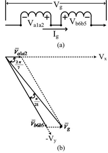
Fig. A.1. (a) Current through the windings of phase voltage  $V_g$ . (b) Phasor diagram of winding voltages.
