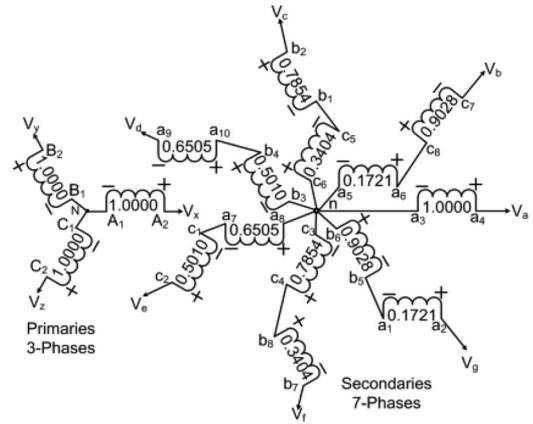
Fig. 1. Proposed transformer winding connection (star).
