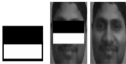
Fig. 5. Detection of eyes using haar features
