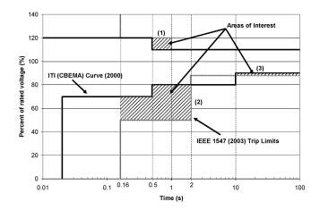
Fig. 2. ITI/CBEMA curve relation to IEEE 1547 trip limits.
