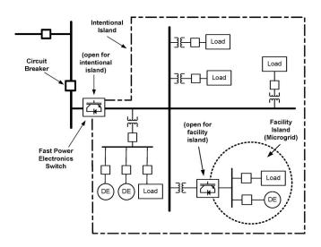
Fig. 4. Intentional island and microgrid example.
