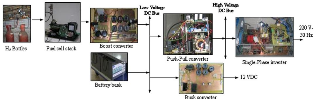
Fig. 10. Simplified scheme with actual systems of the distributed generation system with fuel cell developed.
