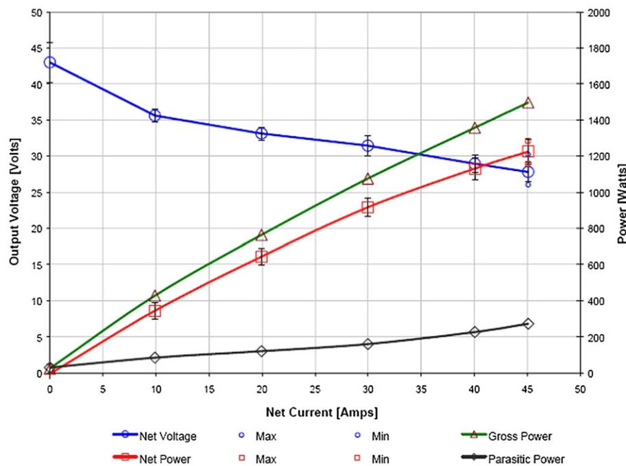
Fig. 6. Polarization and power curves for the Nexa module.
