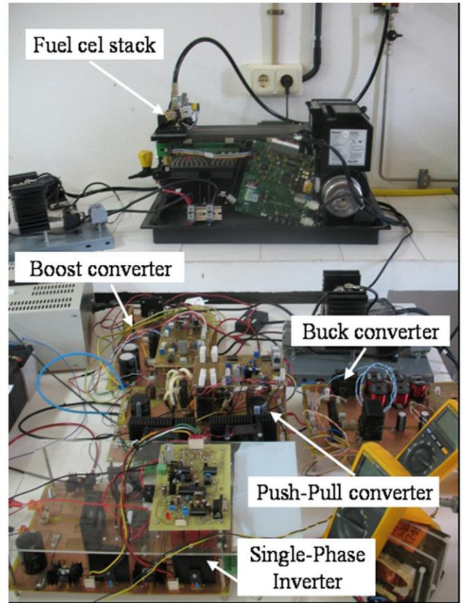
Fig. 11. Distributed generation system with fuel cell developed.
