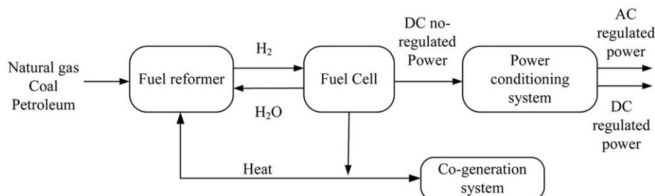
Fig. 2. Fuel cell system basic scheme.
