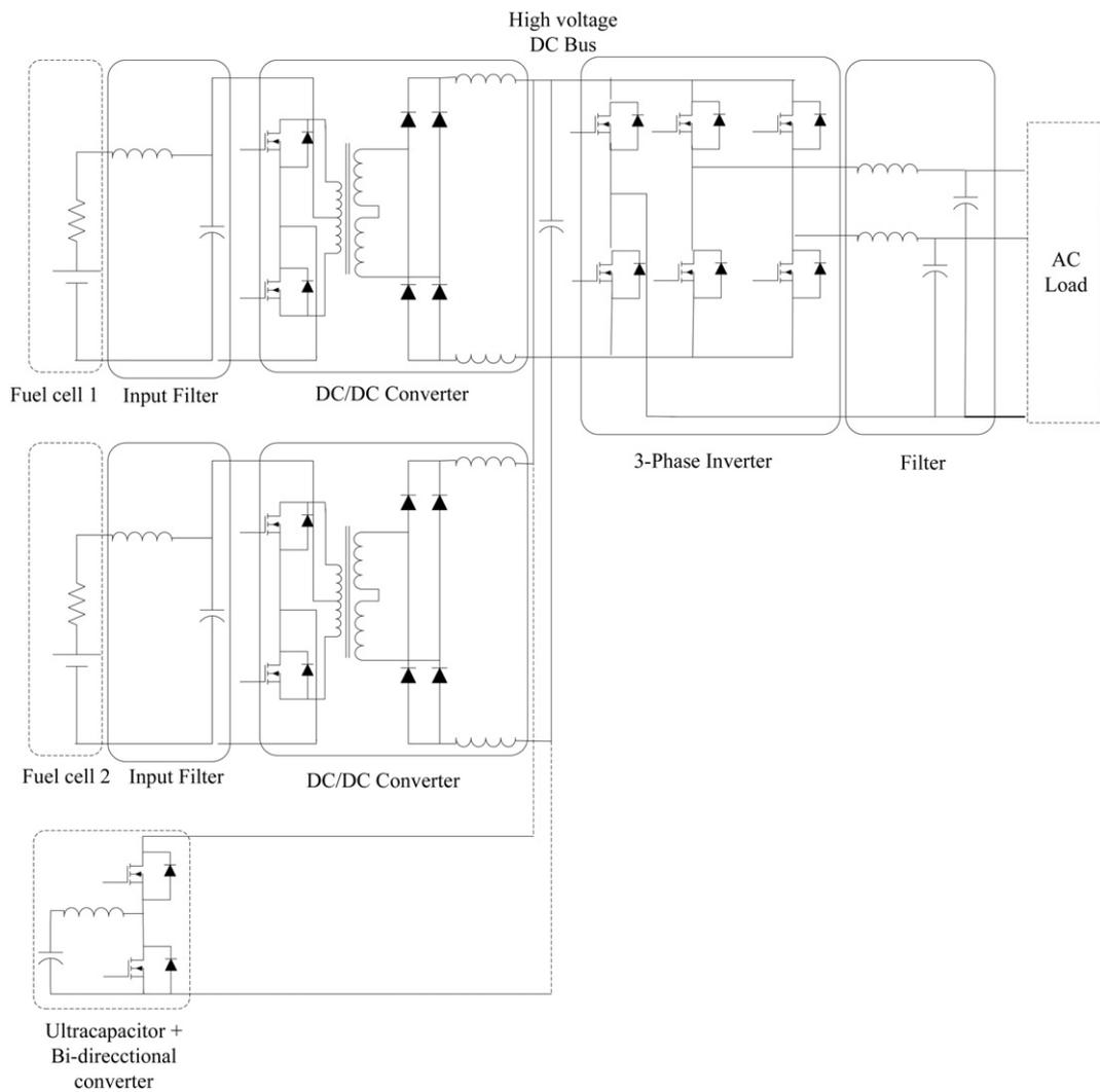
Fig. 4. Circuit topology to supply backup power.
