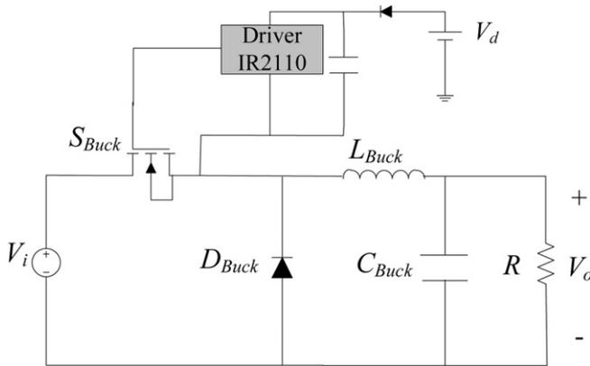
Fig. 8. Bootstrap scheme for Buck converter.
