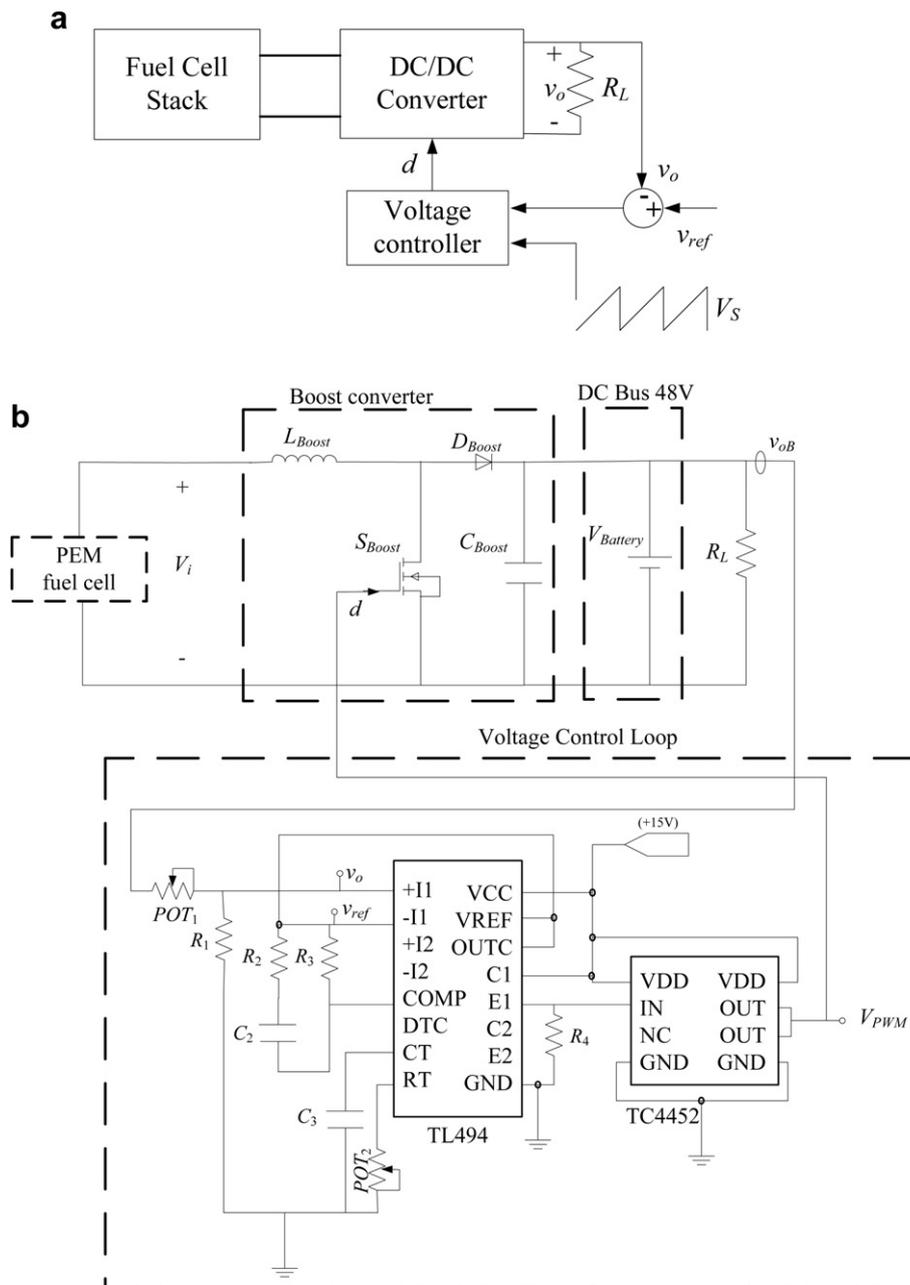
**Fig. 7.** a: Voltage control loop block diagram. b: Scheme of the voltage control loop applied to PEM fuel cell hybrid system.
