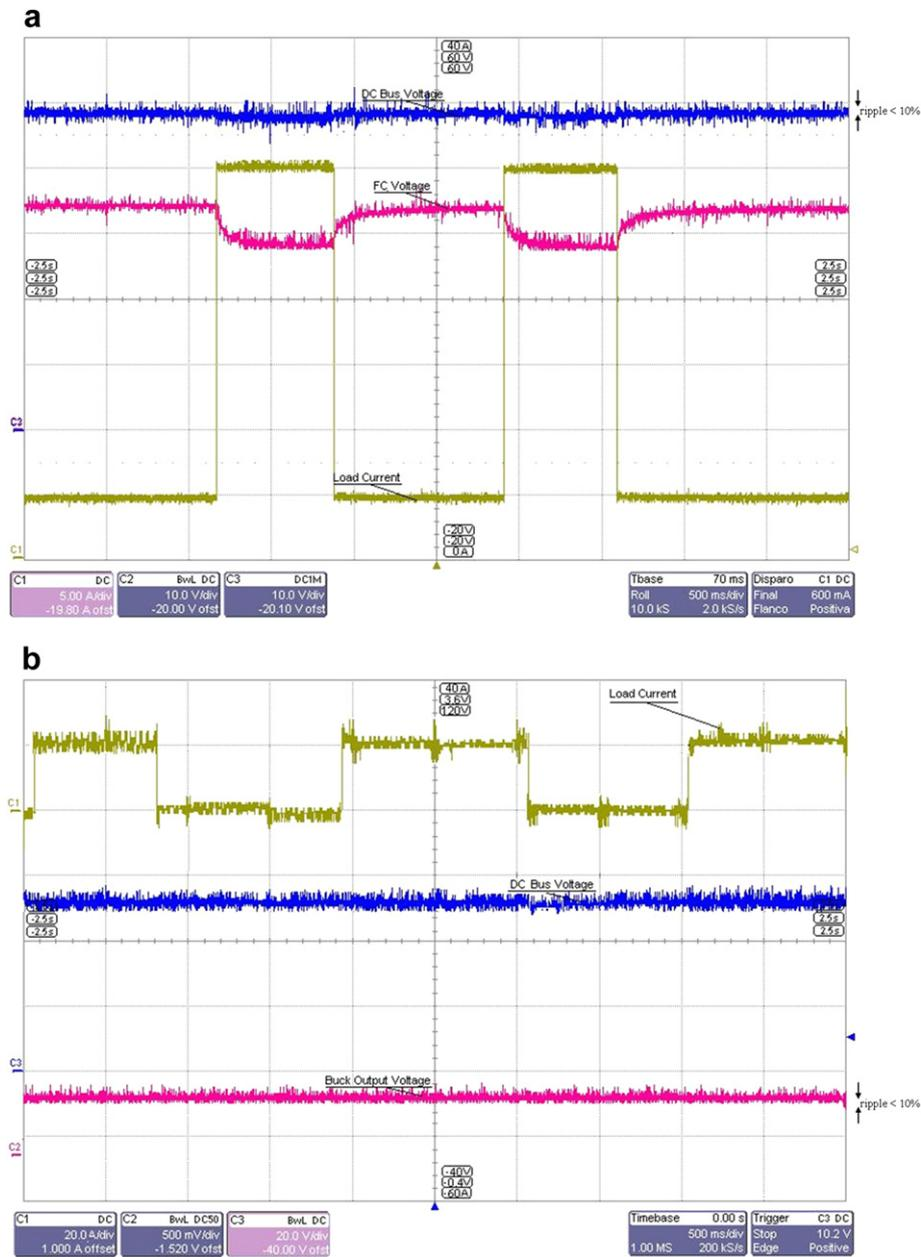
**Fig. 12.** Experimental results when load is connected to DC links. a) Load connected to Low Voltage DC Bus: Load current (Channel C1: 5 A/div, 500 ms/div), Fuel cell voltage (Channel C2: 10 V/div, 500 ms/div), Low DC Bus voltage (Channel C3: 10 V/div, 500 ms/div). b) Load connected to 12 VDC output: Load current (Channel C1: 20 A/div, 500 ms/div), Buck output voltage (Channel C2: 500 mV/div, 500 ms/div, probex20), Low DC Bus voltage (Channel C3: 20 V/div, 500 ms/div).
