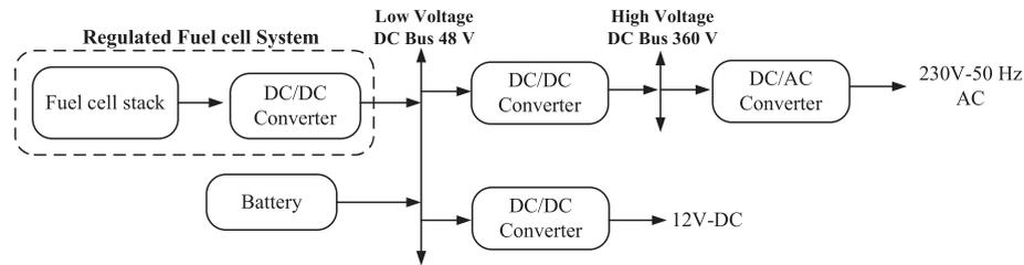
Fig. 1. Backup fuel cell stand-alone hybrid system.
