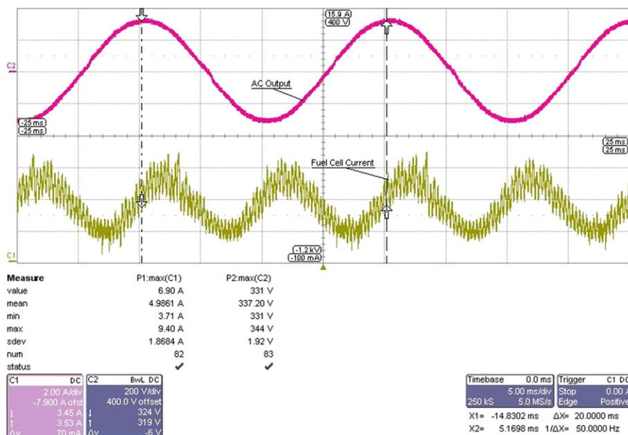
Fig. 15. Experimental results when load is connected to AC Output. Fuel cell current (Channel C1: 2 A/div, 5 ms/div), 230 V-AC Single-phase inverter output voltage (Channel C2: 200 V/div, 5 ms/div).
