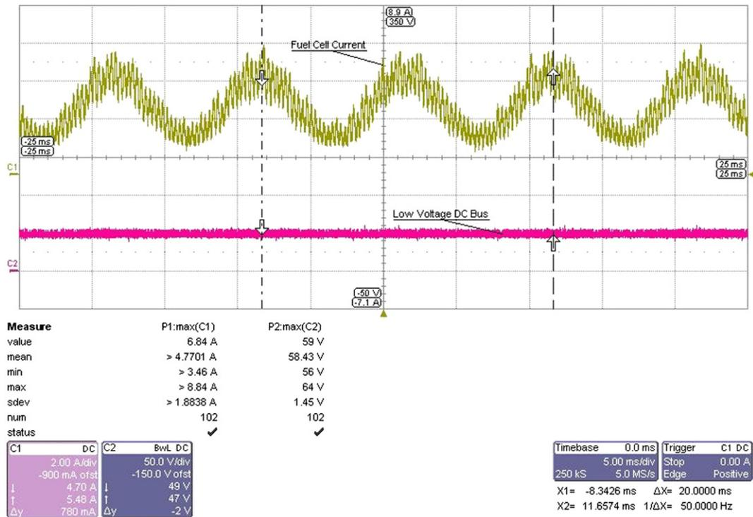
Fig. 13. Experimental results when load is connected to AC Output. Fuel cell current (Channel C1: 2 A/div, 5 ms/div), 48 V-DC Bus voltage (Channel C2: 50 V/div, 5 ms/div).
