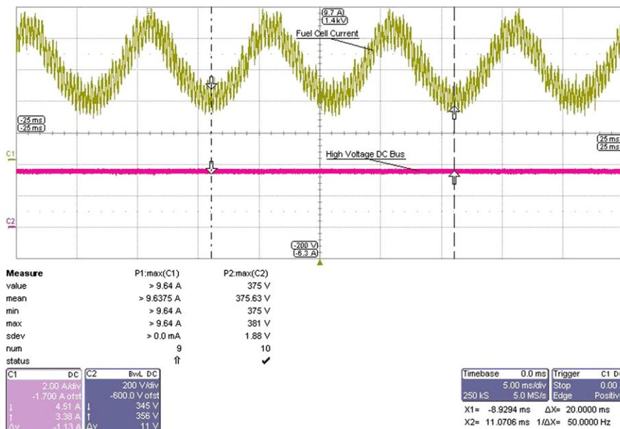
Fig. 14. Experimental results when load is connected to AC Output. Fuel cell current (Channel C1: 2 A/div, 5 ms/div), 360 V-DC Bus voltage (Channel C2: 200 V/div, 5 ms/div).
