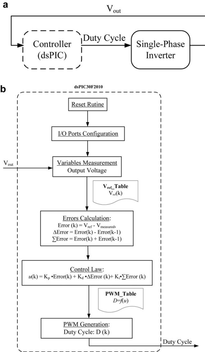
Fig. 9. a: Inverter control scheme implemented. b: Inverter control on dsPIC30F2010.
