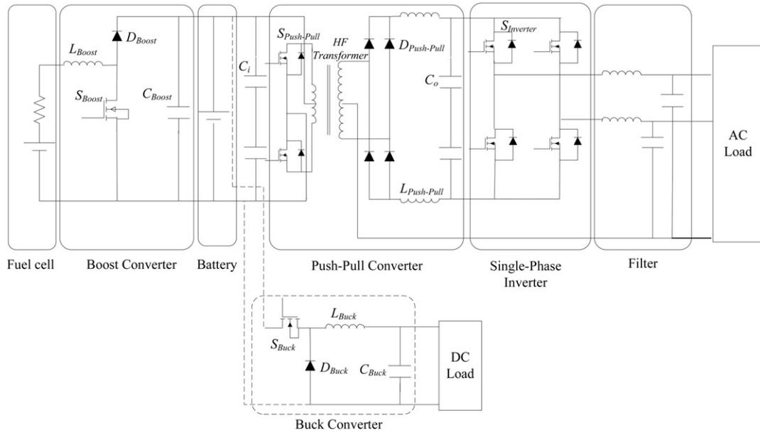
Fig. 3. Circuit topology to supply a dedicated load.
