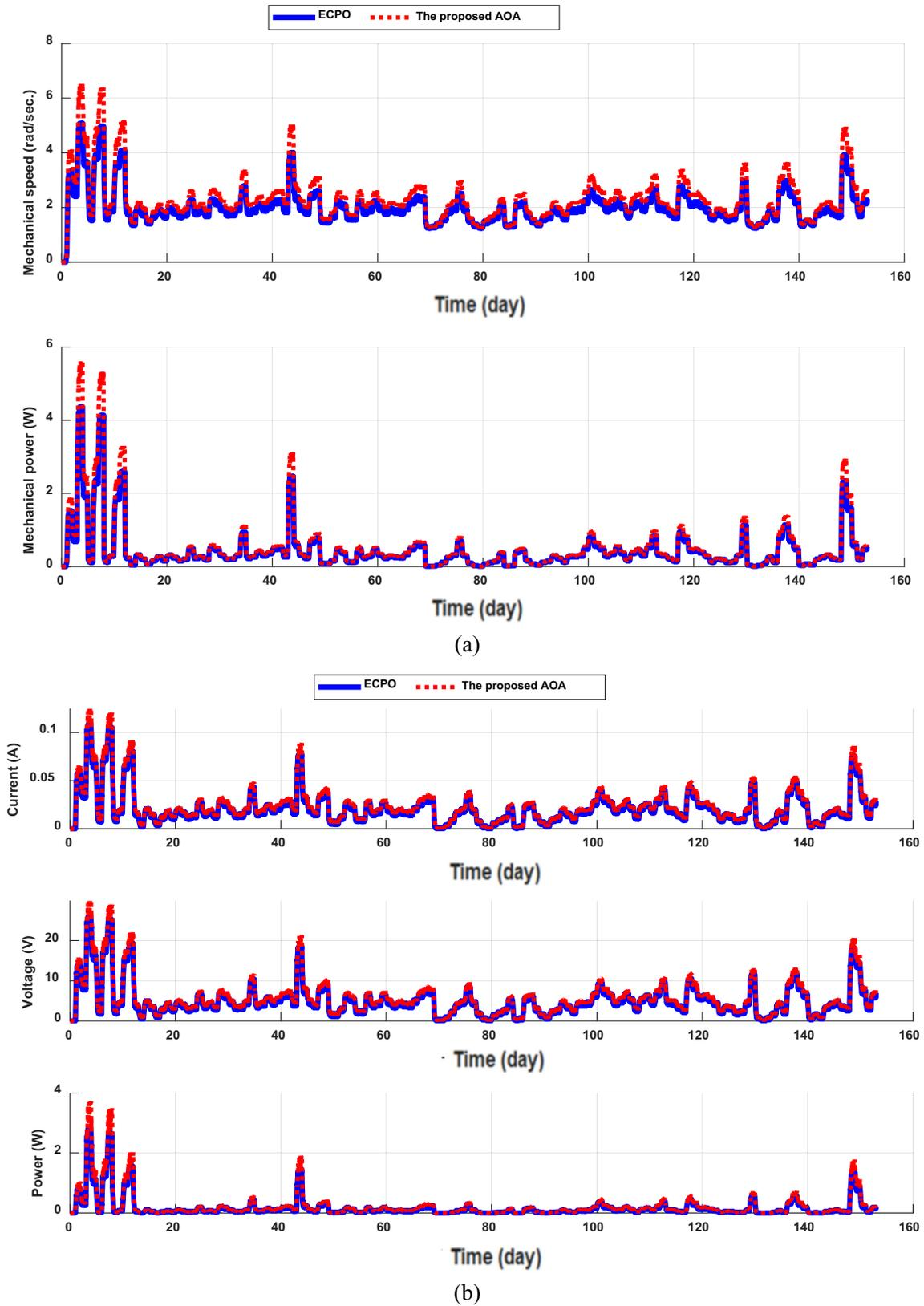
Fig. 17. Time responses of (a) rotational speed and mechanical power, (b) current, voltage, and power for wind generation system installed in Jizan city.
