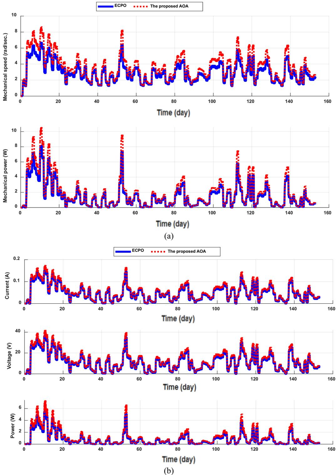
Fig. 15. Time responses of (a) rotational speed and mechanical power, (b) current, voltage, and power for wind generation system installed in Riyadh city.
