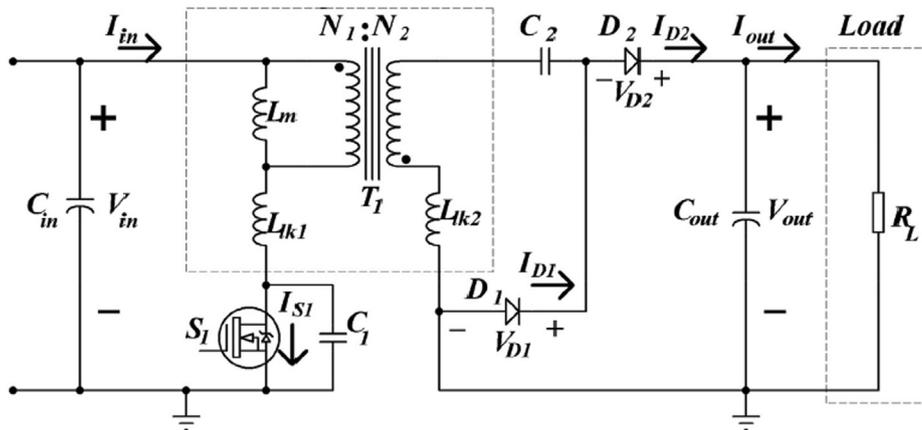
Fig. 4. Equivalent circuit of boost converter [48].
