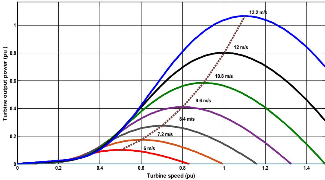
Fig. 3. Mechanical power versus rotational speed.
