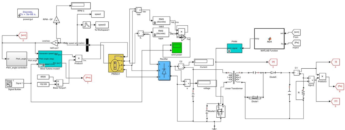
Fig. 7. Simulink model of the proposed AOA-MPPT controller.
