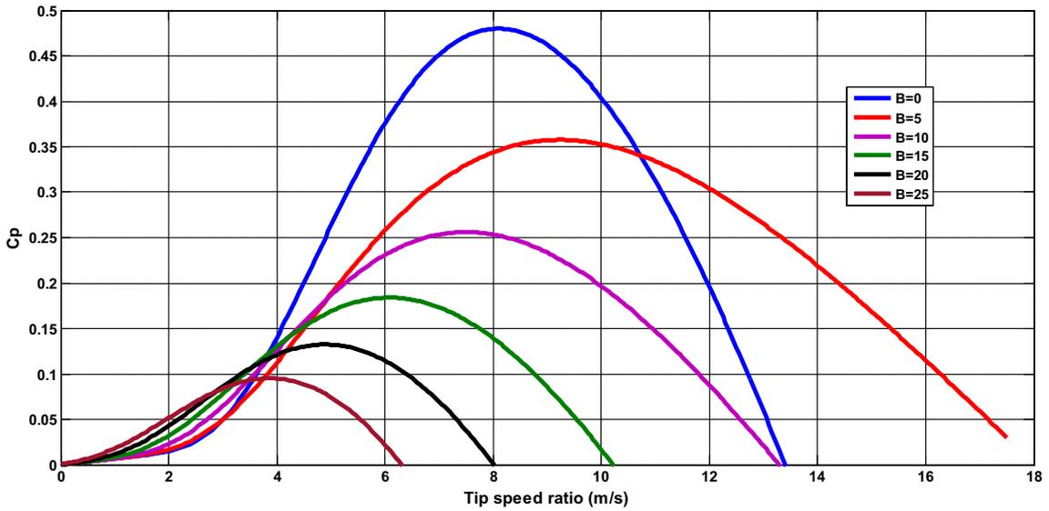
Fig. 2. Variation of  $C_p$  to  $\lambda$  at different  $\beta$ .
