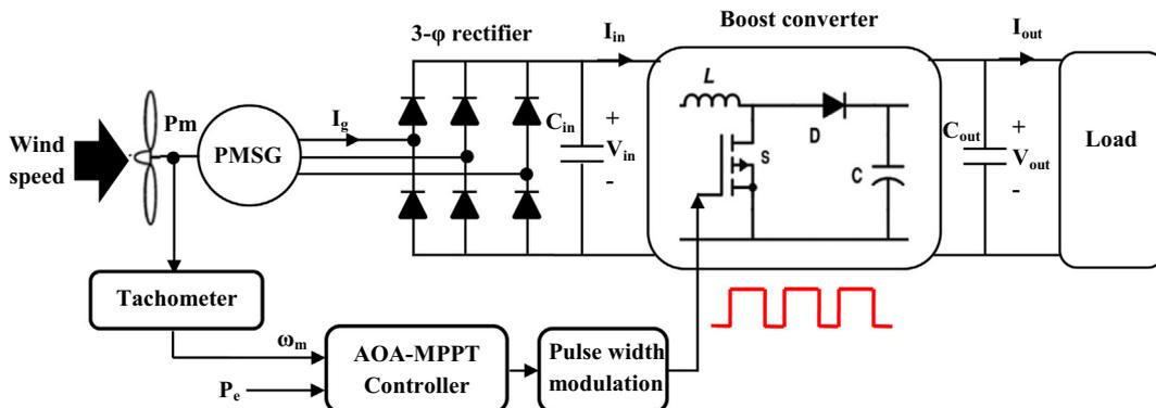
Fig. 1. Construction of wind energy generation system.
