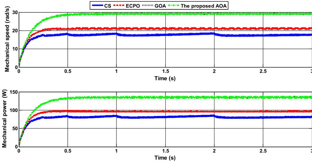
Fig. 9. The time responses of mechanical speed and power at  $V = 12$  m/s.
