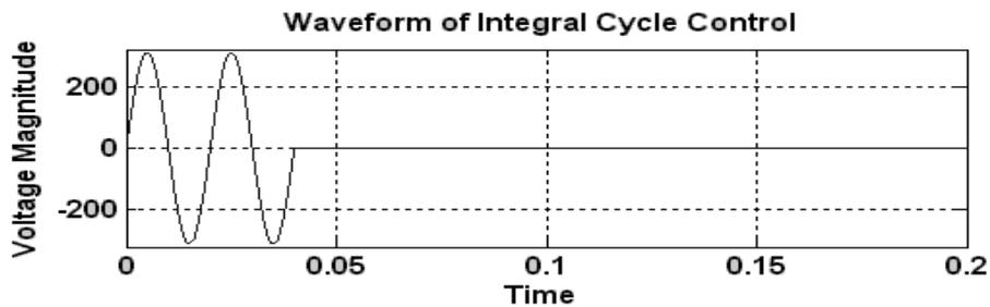
Fig-4: describes the output voltage waveform in ICC with duty cycle  $D = 0.2$  and harmonics
