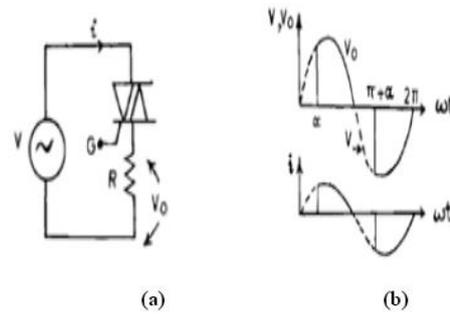
Fig-1(a): Switching arrangement of phase control circuit,
