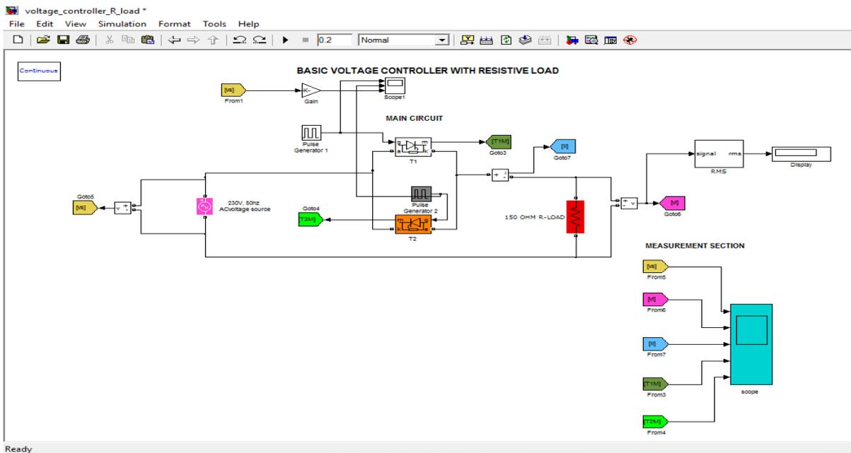
Fig-7: Simulation diagram for Integral cycle switching control
