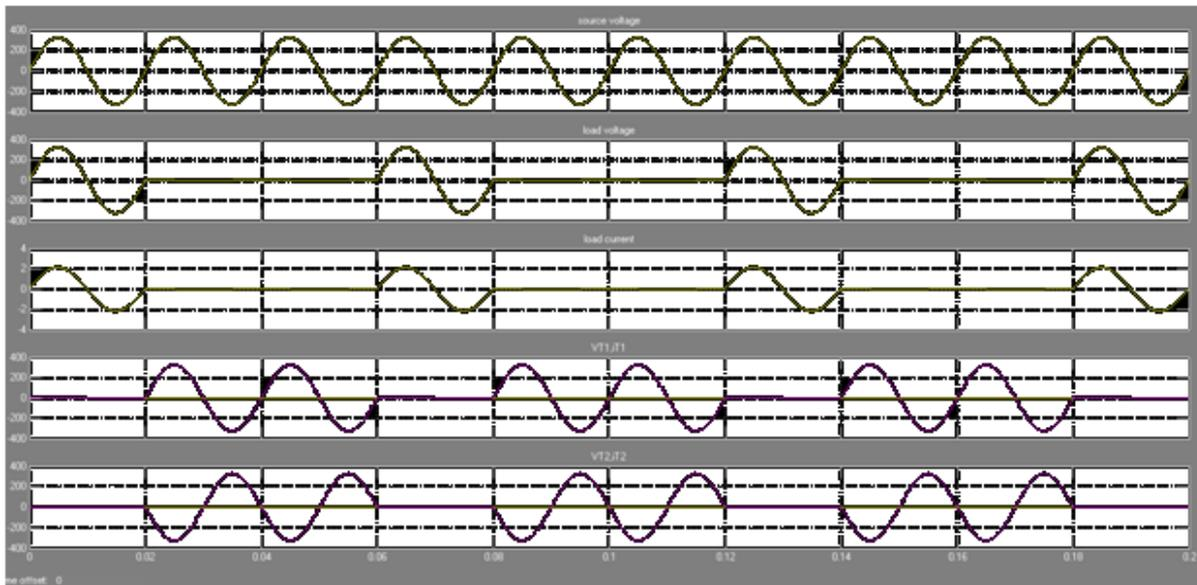
Fig-8: load output voltage and current waveform for firing angle = 30 deg and duty cycle 0.06
