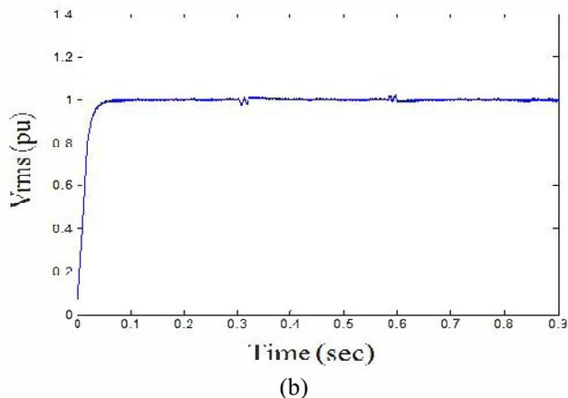
Fig. 7. Voltage  $V_{rms}$  at load point, with line-ground fault: (a) Without DVR and (b) With DVR.
