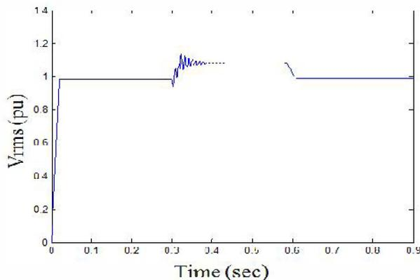
Fig. 10. Voltage  $V_{rms}$  at load point, with three-phase fault, Without DVR.
