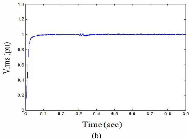
Fig. 5. Voltage  $V_{rms}$  at load point, with three-phase fault: (a) Without DVR and (b) With DVR.
