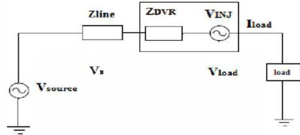
Fig. 3. Equivalent circuit diagram of the DVR.
