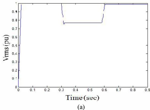
Fig. 9. Voltage  $V_{rms}$  at load point, with line-line-ground fault: (a) Without DVR and (b) With DVR.
