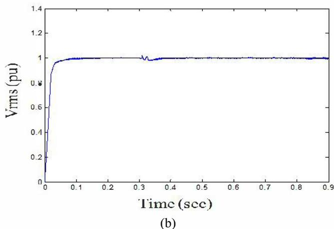
Fig. 6. Voltage  $V_{rms}$  at load point, with three phase-ground fault: (a) Without DVR and (b) With DVR.
