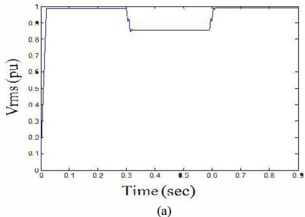
Fig. 8. Voltage  $V_{rms}$  at load point, with line-line fault: (a) Without DVR and (b) With DVR.
