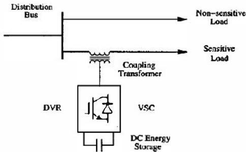
Fig. 2. Schematic representation of the DVR for a typical custom power application.
