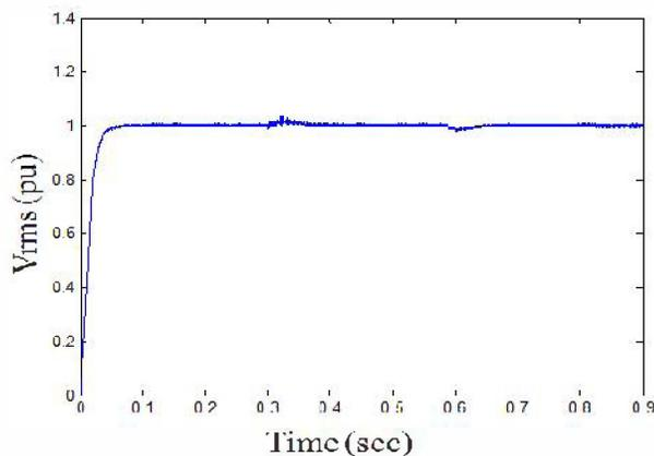
Fig. 11. Voltage  $V_{rms}$  at load point, with three-phase fault, With DVR.
