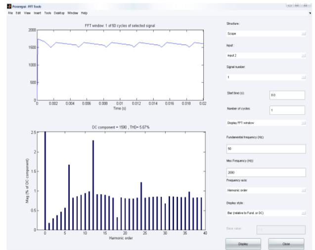
Fig. 5.4. THD for output voltage
