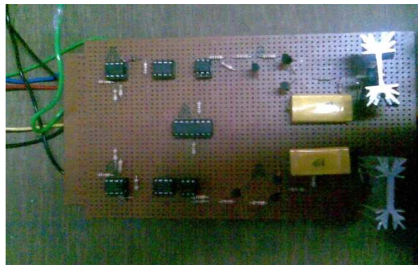
Figure 19. Fabricated single-phase soft starter
