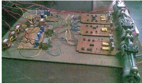
Figure 21. Fabricated three-phase ac voltage regulator using IGBT.
