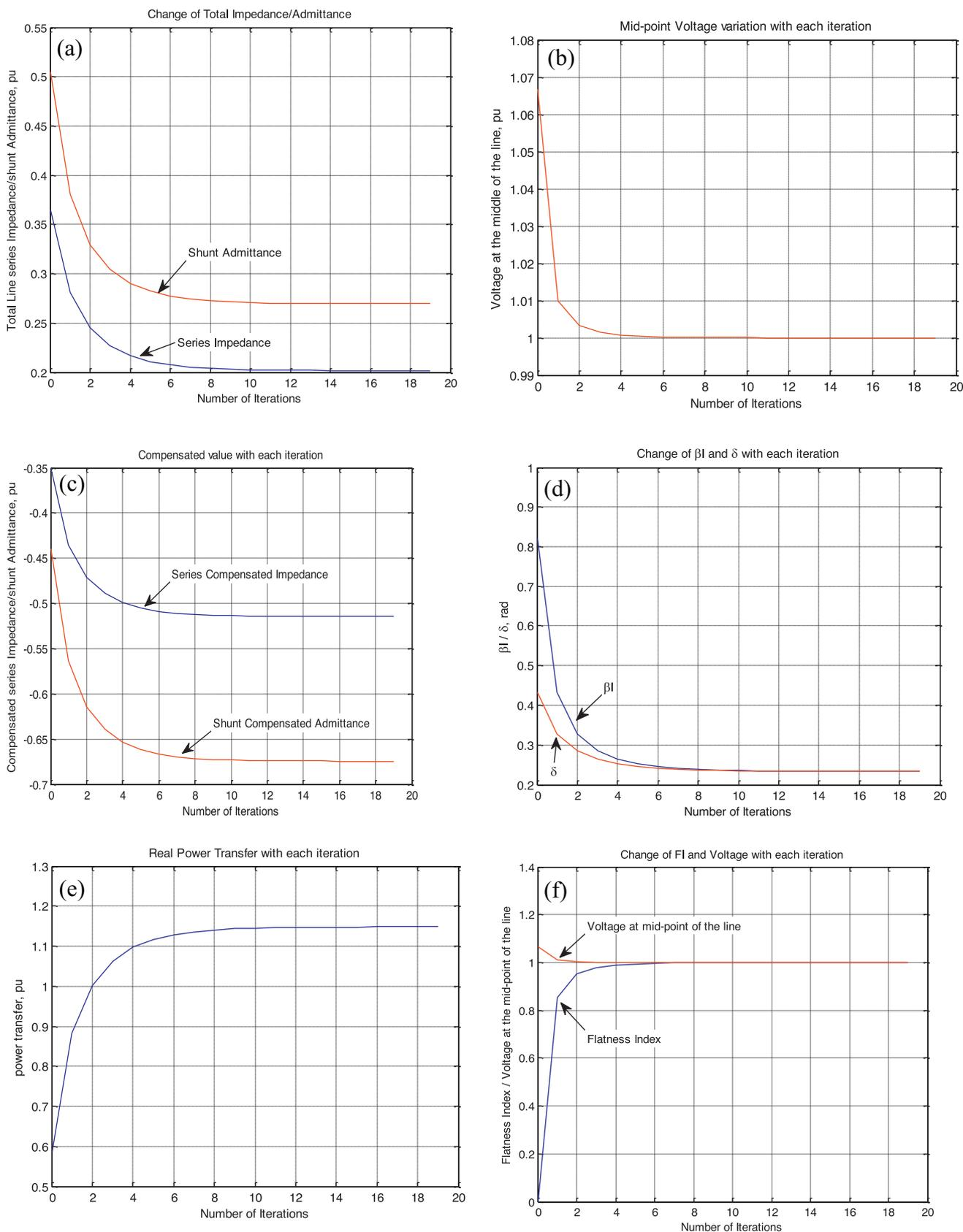
**Fig. 9.** (a) Total line parameters variation. (b) Mid-point voltage variation. (c) Compensator variation. (d)  $\delta$  and  $\beta I$  variation. (e) Variation of real power transfer. (f) Flatness Index variation.
