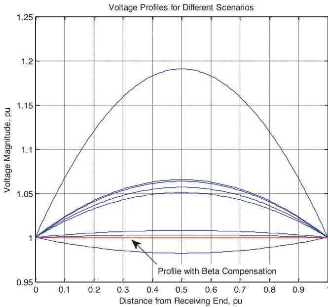
Fig. 10. Voltage profile along the line for different scenarios.
