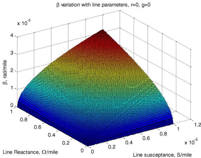
Fig. 4.  $\beta$  variation with line series reactance and shunt susceptance.
