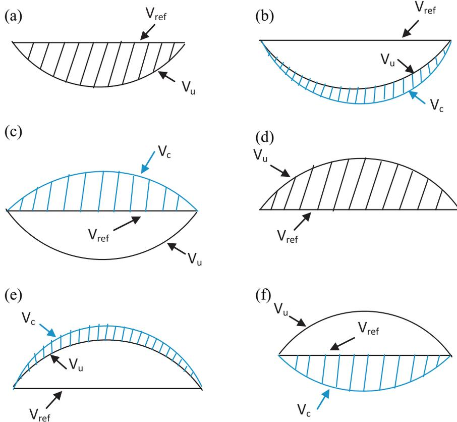
Fig. 7. (a) Voltage profile of sag case with proper compensation. (b) Voltage profile of sag case with improper compensation. (c) Voltage profile of sag case with over compensation. (d) Voltage profile of hump case with proper compensation. (e) Voltage profile of hump case with improper compensation. (f) Voltage profile of hump case with over compensation.
