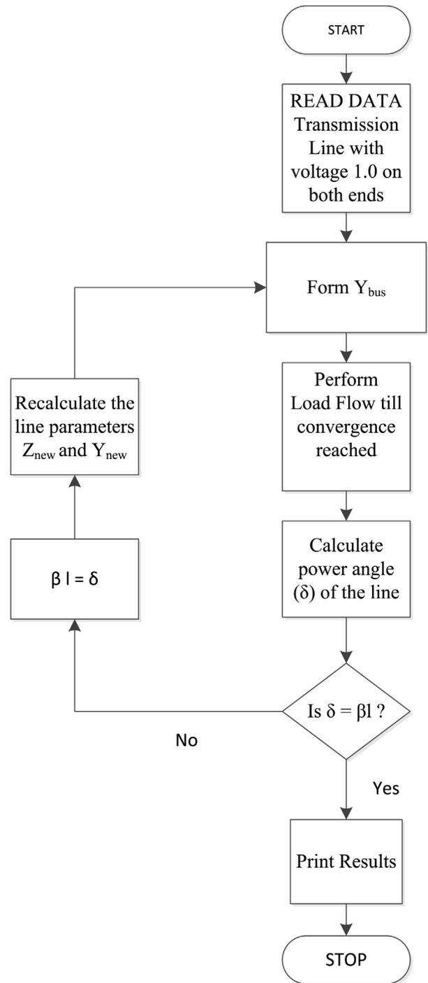
Fig. 5. Flow chart of the beta compensation method.
