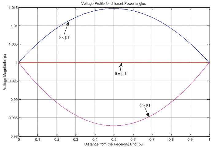
Fig. 3. Voltage profile for different power angles.
