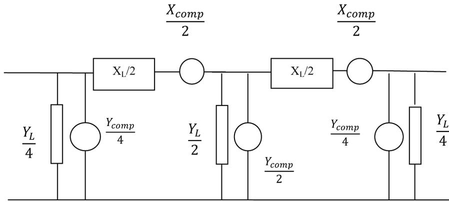
Fig. 6. Equivalent circuit of transmission line with beta compensation.
