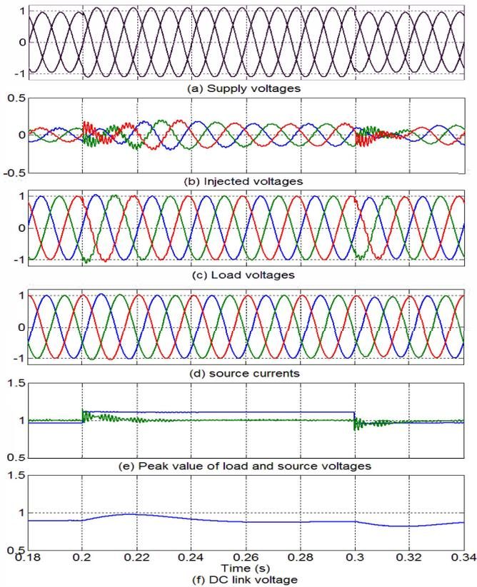
Fig.8 Compensation of balanced voltage swell using DVR.
