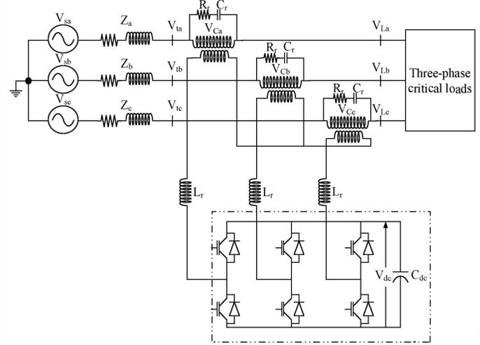
Fig. 3 Schematic diagram of capacitor supported DVR
