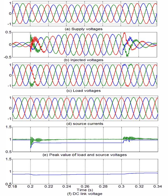
Fig. 7. Compensation of balanced voltage sag using DVR.
