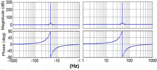
Fig. 5 Bode diagram of an ideal PR controller.
