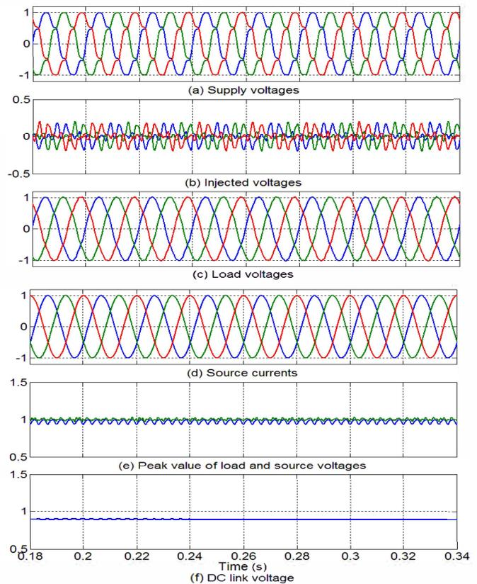
Fig.10 Compensation of harmonics using DVR
