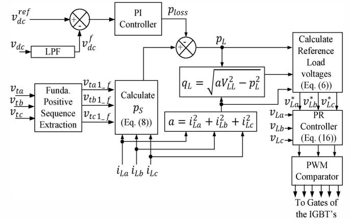
Fig. 4 The complete block diagram of proposed control algorithm.
