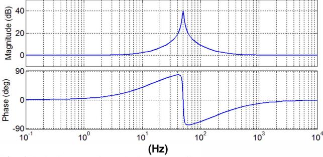
Fig. 6 Bode diagram of practical PR controller.
