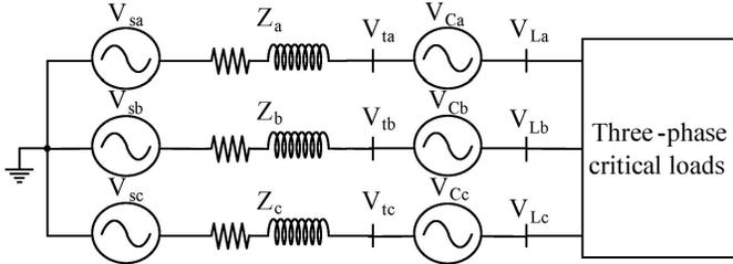
Fig. 1 Schematic diagram DVR connected power system.
