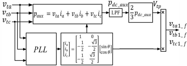
Fig. 2 Proposed fundamental positive sequence extractor
