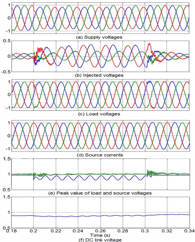
Fig.9 Compensation of unbalanced voltage sag using DVR.
