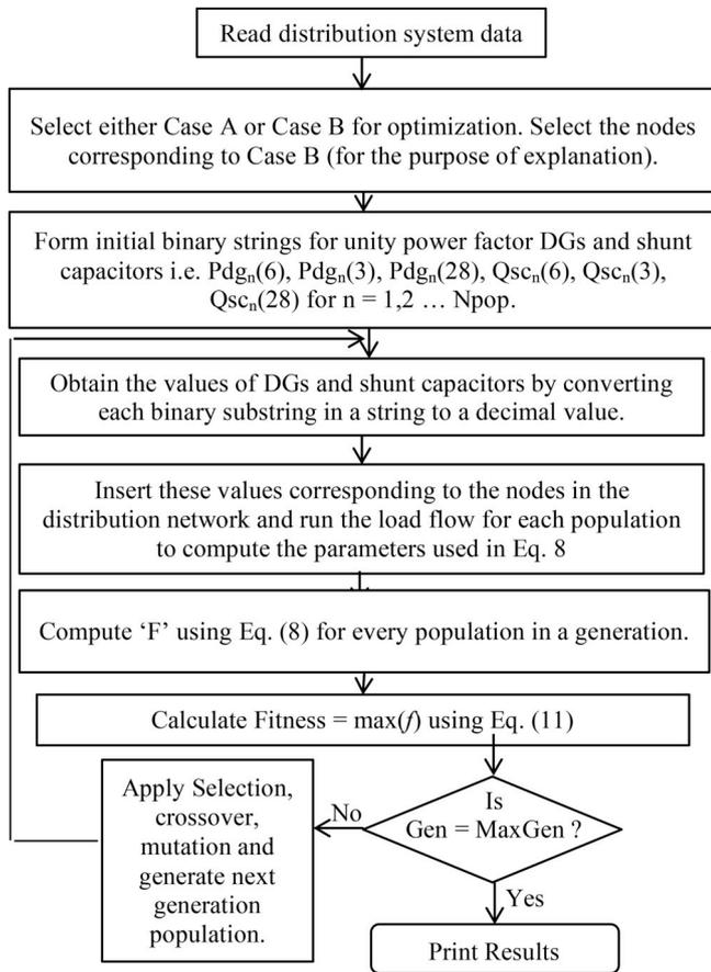
Fig. 5. Flowchart for objective function optimization.
