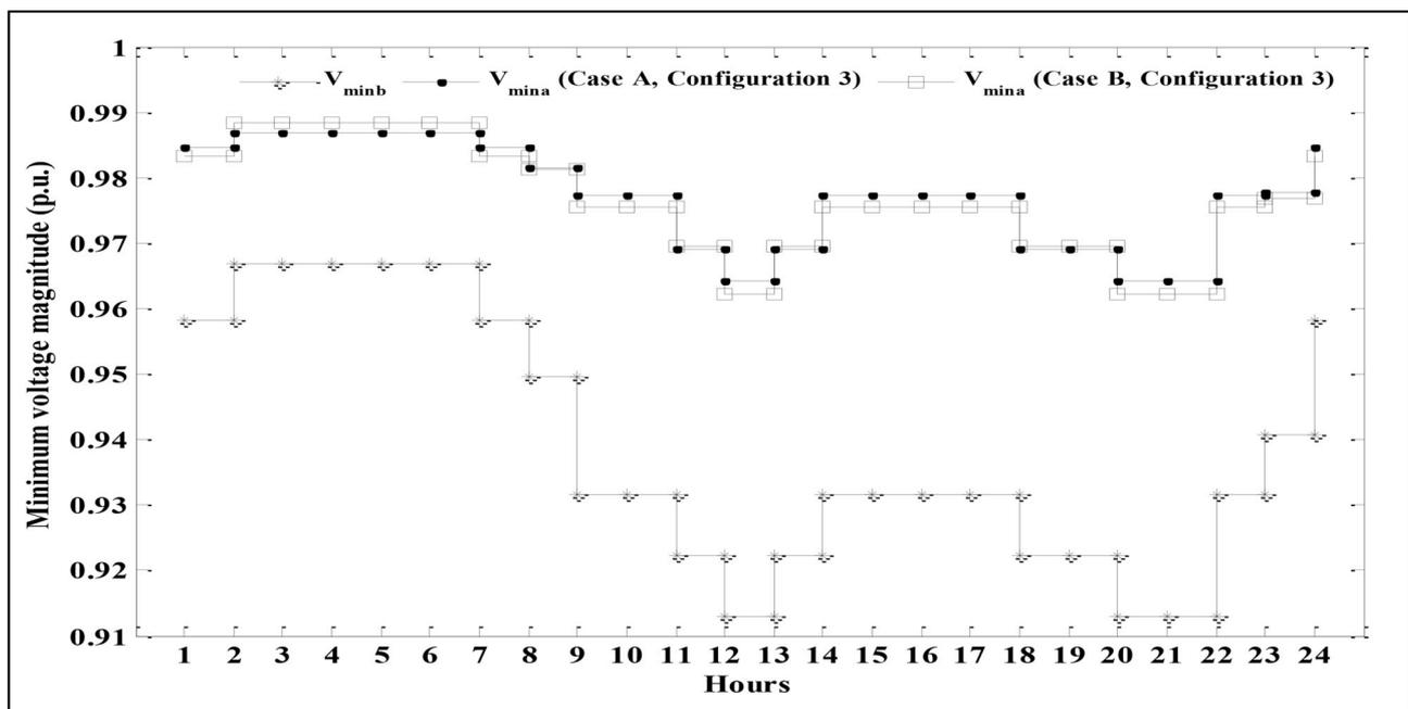
Fig. 6. Graphical representation of minimum voltage magnitude for 24h average daily load schedule.
