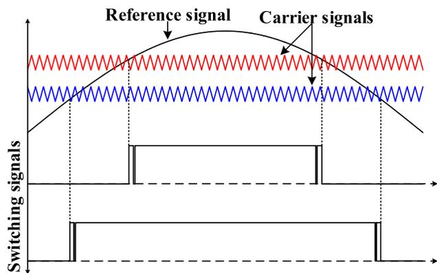
FIGURE 3. Switching pulse generation from the comparison between reference signal and carrier signal.
