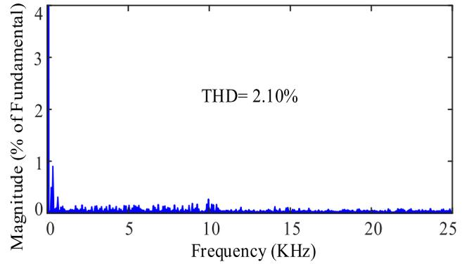
FIGURE 18. Frequency spectrums of the output line voltage.
