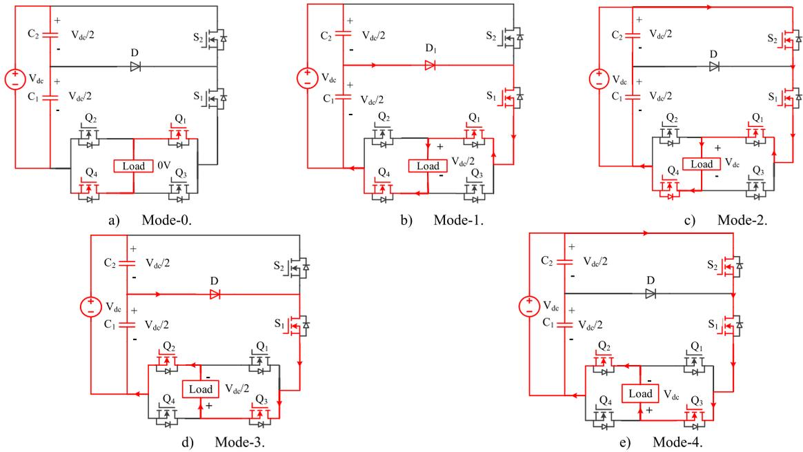
FIGURE 4. Five operating modes of the proposed 5-level inverter unit (single phase).
