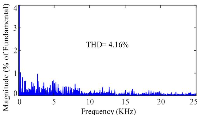
FIGURE 14. Frequency spectrums of the output line voltage.
