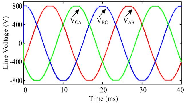
FIGURE 15. Output line voltage of the 39-level inverter (3-Ø).
