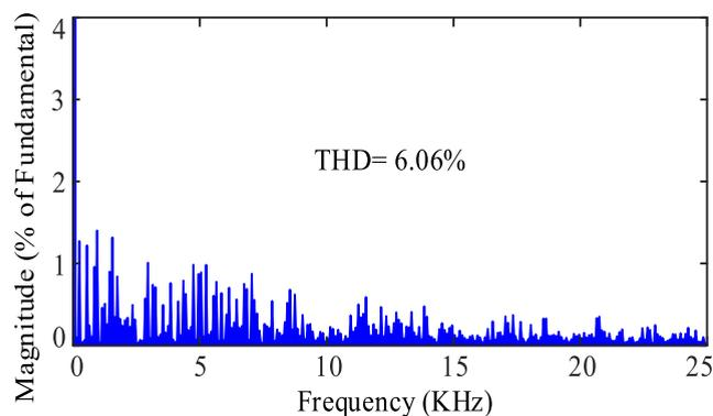
FIGURE 10. Frequency spectrums of the output line voltage.
