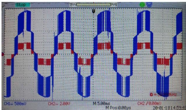
FIGURE 25. Unity power factor characteristics verification of the prototype.
