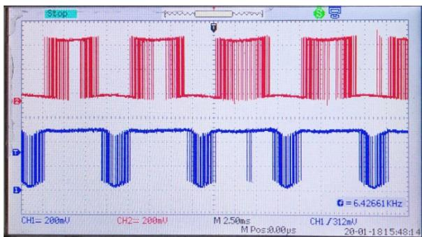
**FIGURE 20. Switching pulses of S1 (lower) and S2 (upper) switches.**
