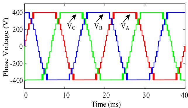
FIGURE 12. Output phase voltage of the 13-level inverter (3-Ø).
