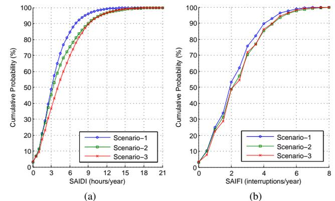
Fig. 12. Cumulative probability distributions of (a) SAIDI and (b) SAIFI with a capacity factor of 30% for wind and solar PV based DG units
