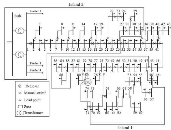
Fig. 9. Island formations due to the faults at branch 1-2 and branch 32-33
