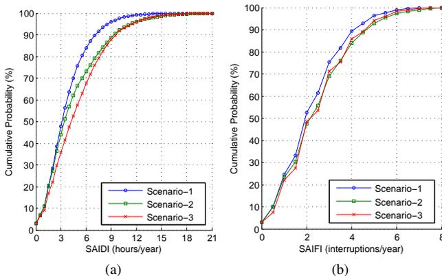
Fig. 11. Cumulative probability distributions of (a) SAIDI and (b) SAIFI with a capacity factor of 20% for wind and solar PV based DG units
